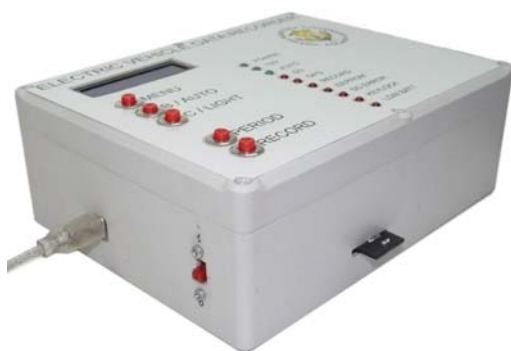
Fig.3. The EVDR enclosure with SD card socket, ON/OFF switch and USB power cable
