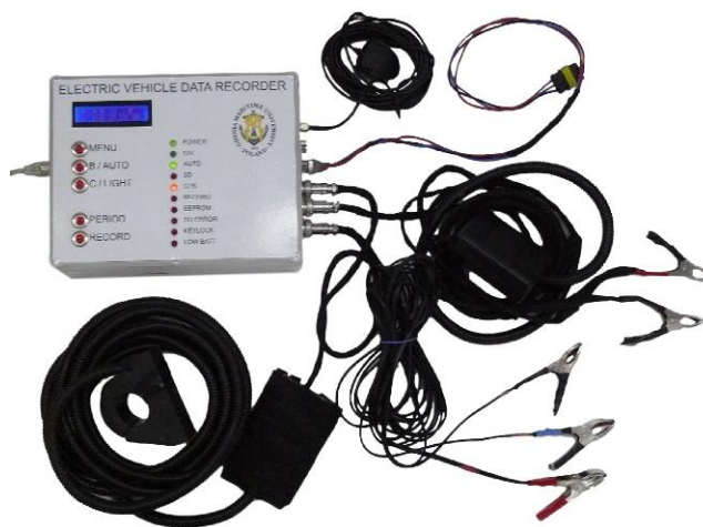
Fig.1. Electric Vehicle Data Recorder with assortment of probes.
