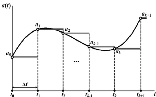
Fig.1. The sequence the reading of vibration acceleration values  $a(t)$
