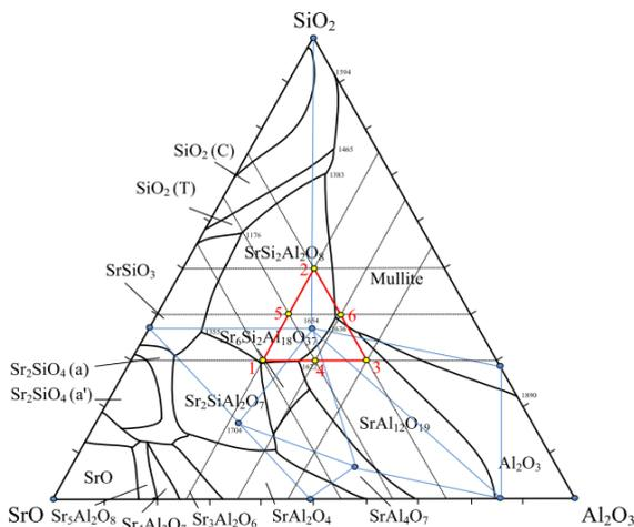
Fig.1. Location of simplex-lattice plan on ternary system SrO–Al<sub>2</sub>O<sub>3</sub>–SiO<sub>2</sub>
