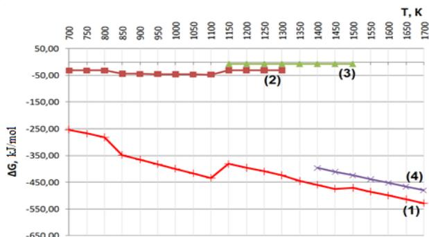
Fig.3. Gibbs energy for the reactions 1-4 for reference point of simplex-plan in a temperature range 700–1700 K
