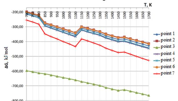
Fig.2. Graphic dependency of the ΔG, kJ/mol for strontium anorthite that was obtained from oxide (according to reaction 1)
