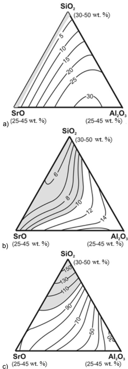
Fig.4. "Composition – property" dependencies for developed compositions of radio transparent ceramics, sintered at temperature 1350°C: a) water absorption ( $W$ , %); b) dielectric permittivity ( $\epsilon$ ); c) compression strength ( $\sigma_{\text{compression}}$ , MPa)
