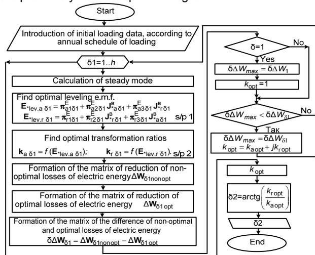
Fig.2. Block diagram of the algorithm for determining the optimal angle CT optimal branch
