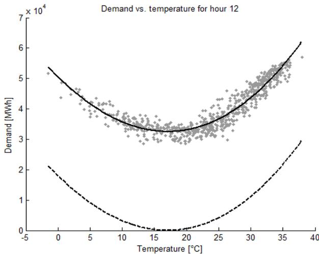
Figure 1. Example of weather-related component extraction [6] applied to one of datasets: interpolated curve (solid line) and shifted curve representing weather component (dashed line)
