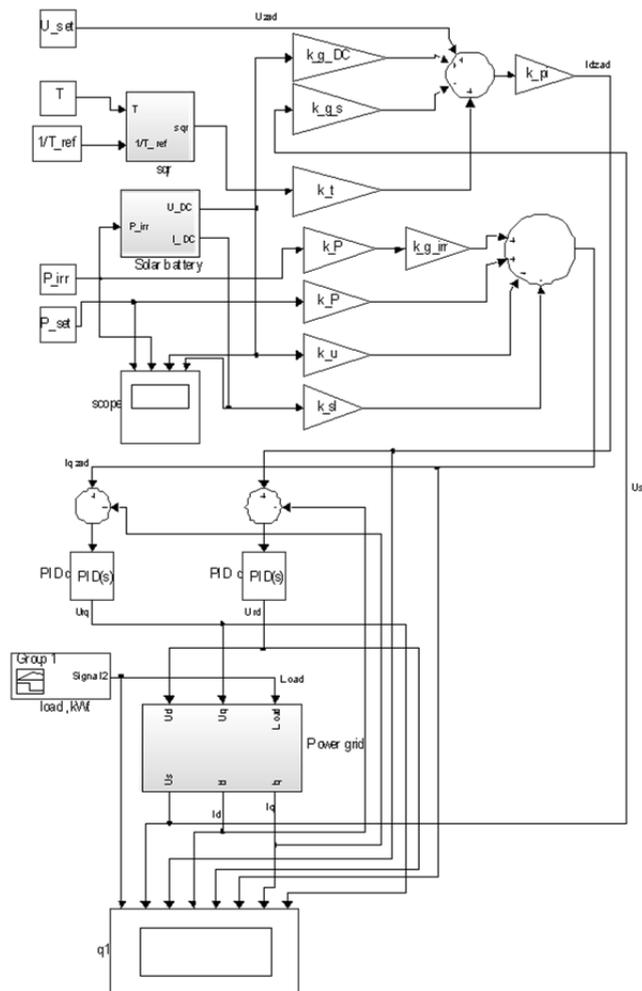
Fig.10. The computer model to test the adequacy of control of  $d$  and  $q$  current components of power inverter:  $sqr$  - square value ratio of temperature solar cell to the temperature difference between solar battery and environment
