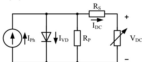
Fig.1. An equivalent electric circuit of solar battery
