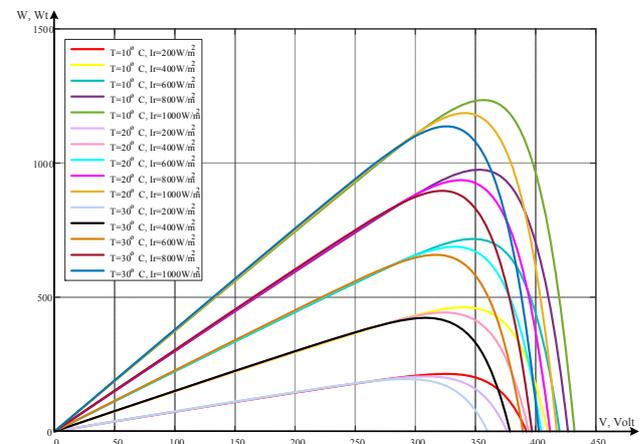
Fig.4. Graph of power relationships, which may be produced by a solar module to grid inverter during the operation with the actual output voltage at difference values of temperature of the solar module
