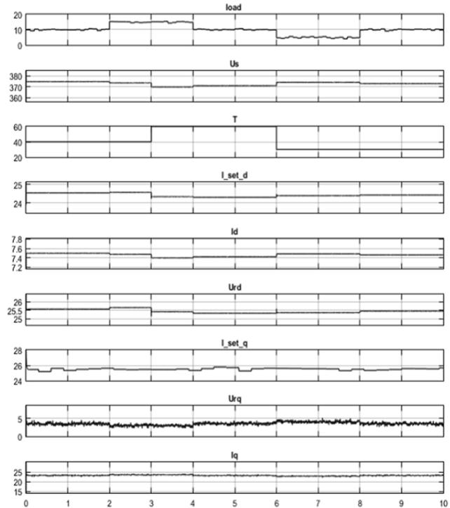
Fig.11. Simulation results for PID controllers of longitudinal and transverse components of the current inverter according to (17)
