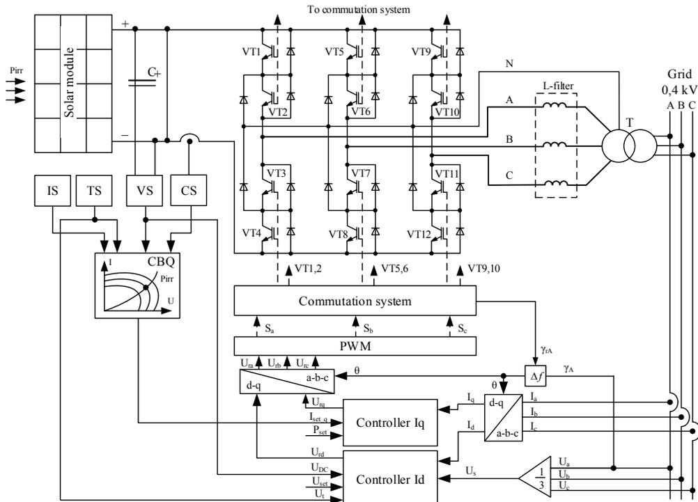
Fig.5. Chain diagram of three level grid inverter with internal circuits for regulation of currents  $I_d$  and  $I_q$ ; IS – illumination sensor; TS – temperature sensor, VS – voltage sensor, CS – current sensor
