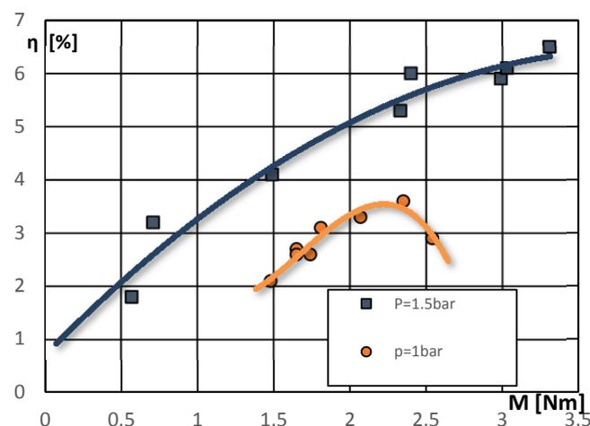
Fig.5 Characteristic of efficiency relative to the torque on motor shaft
