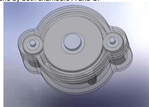
Fig.2 Prototype of pneumatic motor
