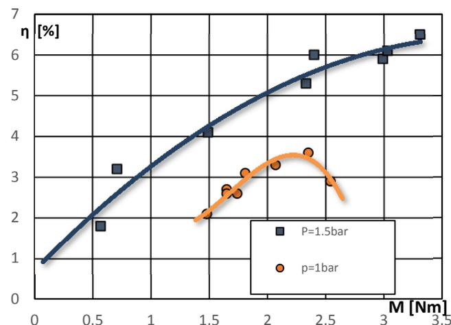
Fig.5 Characteristic of efficiency relative to the torque on motor shaft
