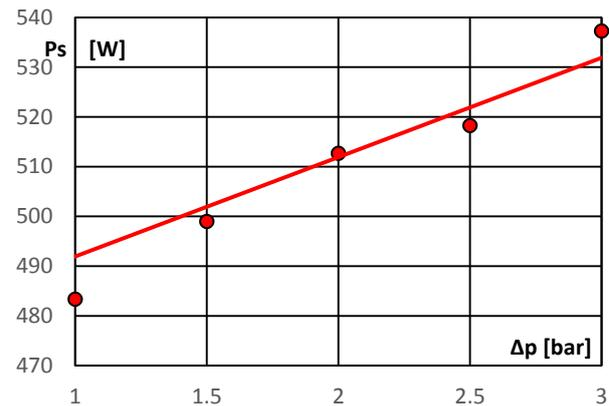
Fig.6 Power of the motor shaft
