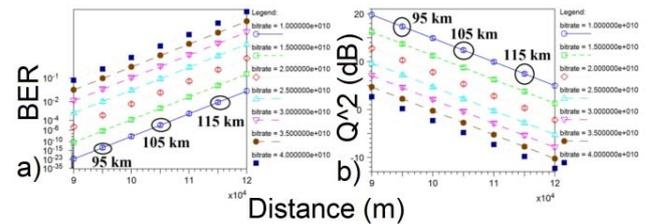
Fig.6. BER and Q-factor dependent on the length of the fibre and bit speed
