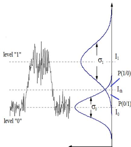
Fig.3. Received optical signal with marked noise dispersion [8]
