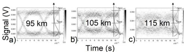
Fig.5. Eye diagrams for 95 km, 105 km and 115 km
