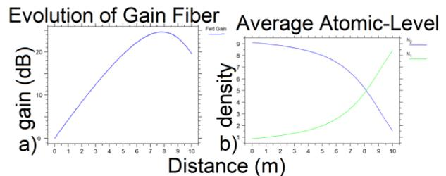
Fig.7. Distance with gain and excited erbium state for EDFA
