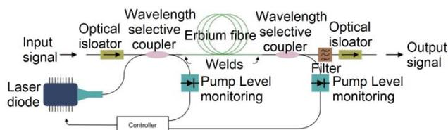
Fig.2. Scheme of EDFA connection
