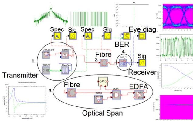
Fig.4. Topology of the optical line with the speed of 10 Gbps
