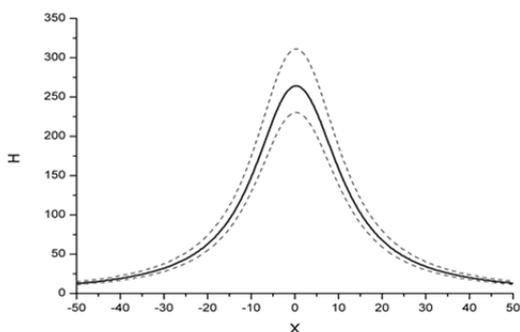
Fig. 4. Distributions of the magnetic field below the line in Fig. 2 corresponding to the constant current during the measurement (continuous line) and its extreme values (dotted lines)
