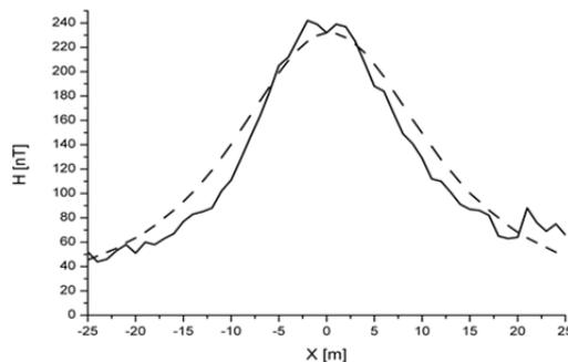
Fig. 5. Magnetic field distribution obtained by the measurement (solid line) and the calculation method (broken line)
