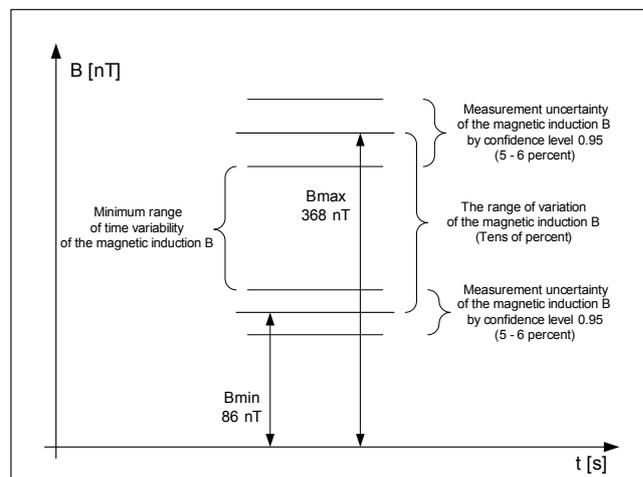
Fig. 6. Graphical presentation of the range of variation of the magnetic induction and measurement uncertainty for a confidence level of 0.95
