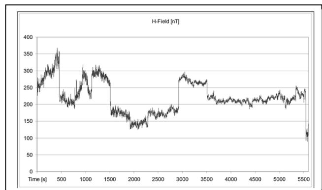
Fig. 3. The course of changes in the measured value of magnetic field under the 110 kV line for B2 pylons in the city of Wrocław
