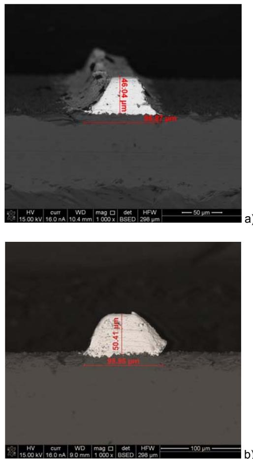
Fig. 2. The SEM micrographs of a cross section of solar cell contacts obtained by technique: a) stencil printed – the squeegee blade with hardness of 80A and b) stencil printed – the squeegee blade with hardness of 95A
