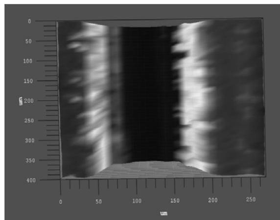
Fig. 3. The light beam induced current (LBIC) map obtained by a 20 mW diode laser with spot resolution of about 10  $\mu\text{m}$  for the grid line of the Stencil – 95A cell
