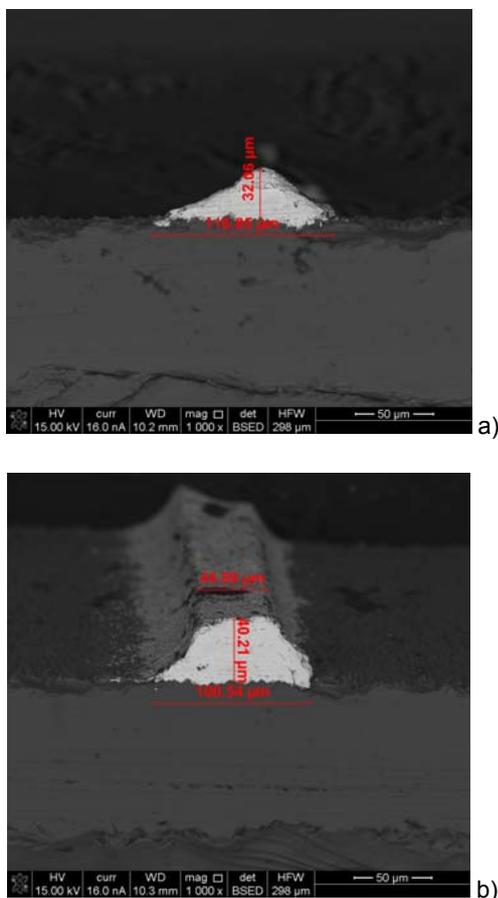
Fig. 1. The SEM micrographs of a cross section of solar cell contacts obtained by technique: a) a screen printed, b) stencil printed, by applying the squeegee blade with hardness of 65A
