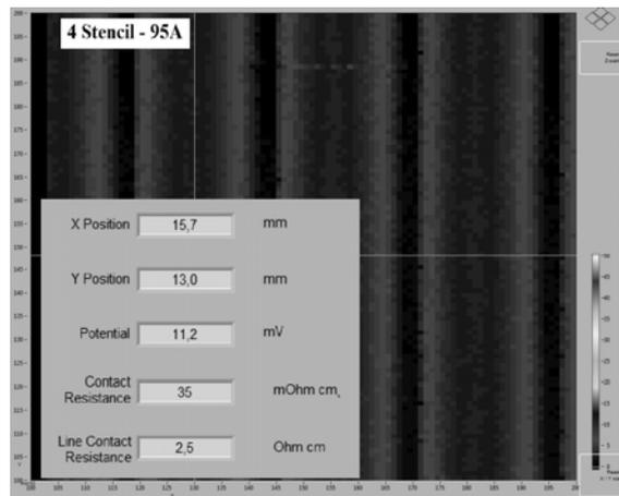
Fig. 4. The 2D representation of contact resistance measurement result with the Corescanner of Stencil – 95A cell.
