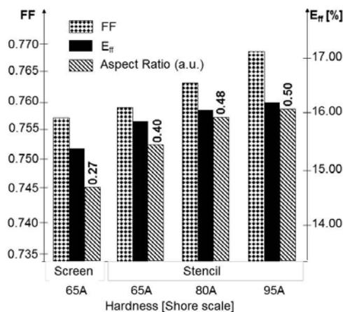
Fig. 5. The dependence of fill factor, solar cell efficiency and aspect ratio on hardness of the used squeegee blades in stencil printing process. For comparison, the parameters of the screen printed solar cell are enclosed also.
