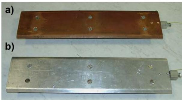
Fig.16. Layer type secondary a) copper, b) aluminum
