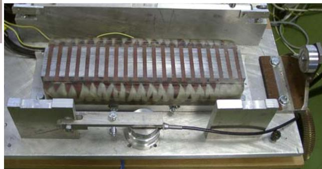
Fig.18. Device for driving and normal forces measurement
