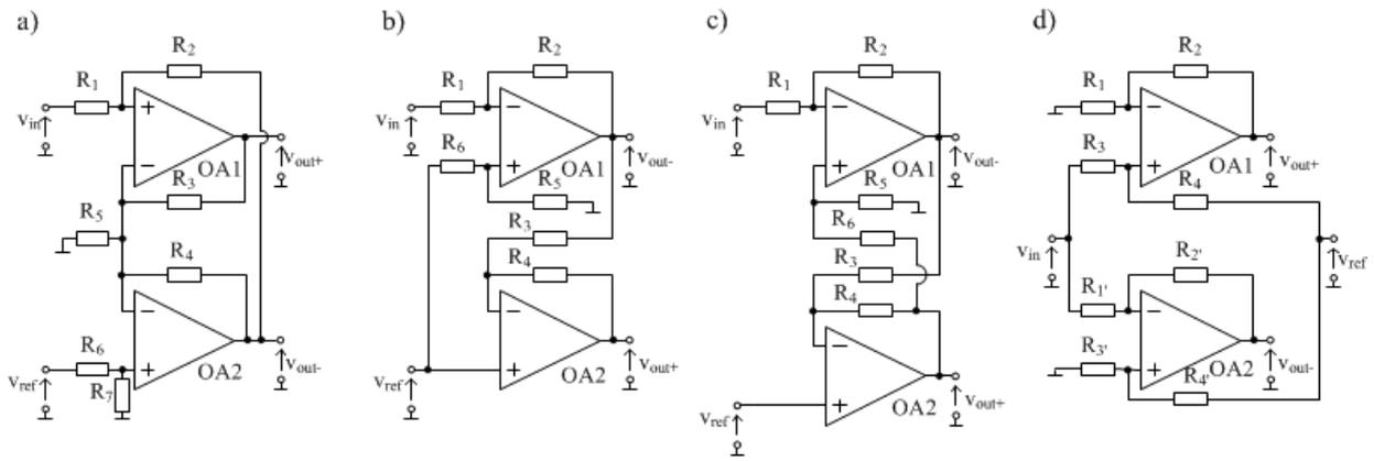
Fig. 2. Op-amp based implementations of single-ended to differential converters
