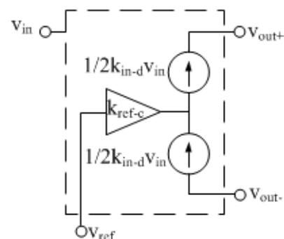
Fig. 1. A functional diagram of a single-ended to differential converter.
