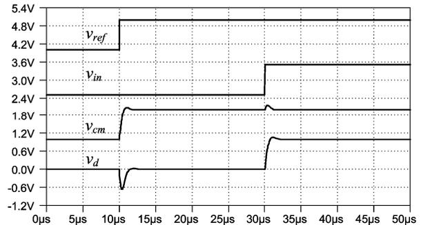
Fig. 4 Step response of the converter – differential-mode and common-mode
