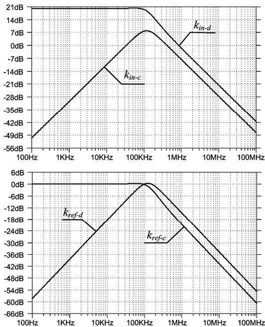
Fig. 3. Frequency response of the converter (simulation results)
