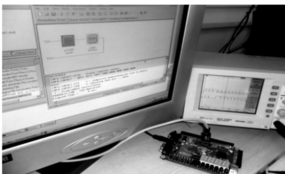
Fig.8. Photograph of the control signals generated by the FPGA based on PMPWM using 2D addressing mode
