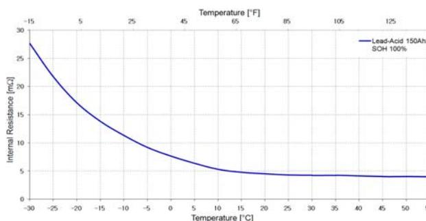
Fig.8. Temperature dependence of internal resistance of a 150Ah Lead-Acid battery (rated current 1C)
