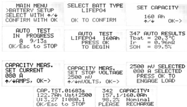
Fig.9. View of EVBT screens of battery setup, auto test and capacity test functions
