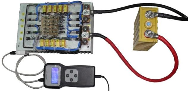
Fig.3. Electric Vehicle Battery Tester during SOH determination of a LiFePO4 battery
