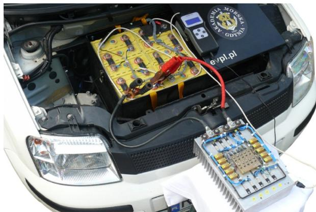
Fig.6. Electric Vehicle Battery Tester during test of the battery pack in a Fiat Panda EV car
