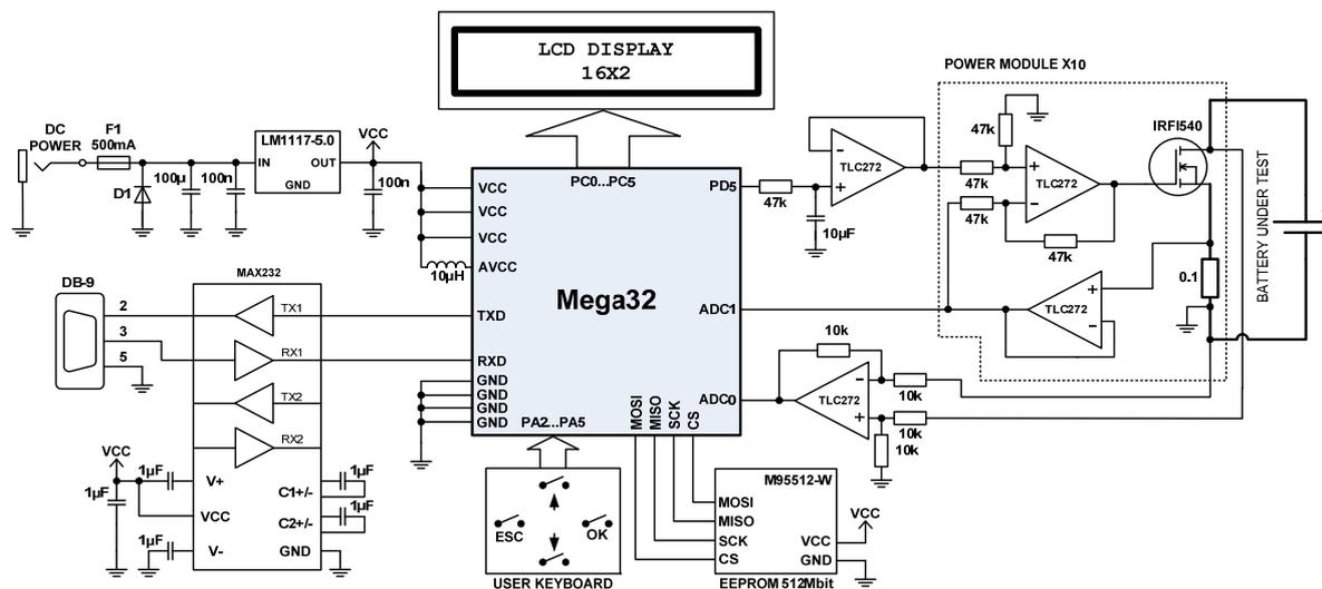
Rys.2. Electric Vehicle Battery Tester schematic diagram
