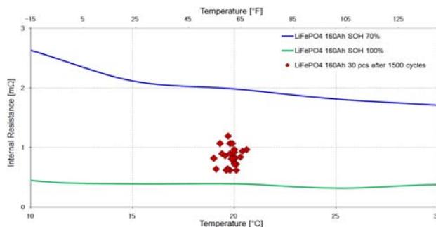
Fig.7. Temperature dependence of internal resistance of a 160Ah LiFePO4 battery (1C rated load current)
