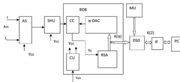
Fig.2. Structural diagram of system of digital processing of analog signals
