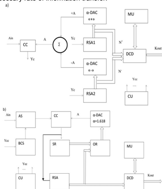
Fig.1. Structural diagrams of bitwise self-calibrated ADC of accelerated speed with weight redundancy on the base of: a) CSWR (1, 1); b) CSWR (0, 1)
