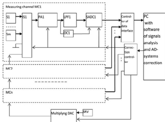
Fig.3. Structure of multichannel AD-system of acoustic sensors signals analysis with the correction of measuring channels characteristics
