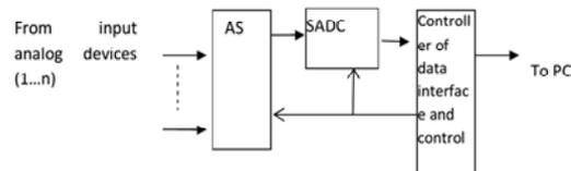
Fig.4. Variant of the circuit with serial AD-conversion of channel signals
