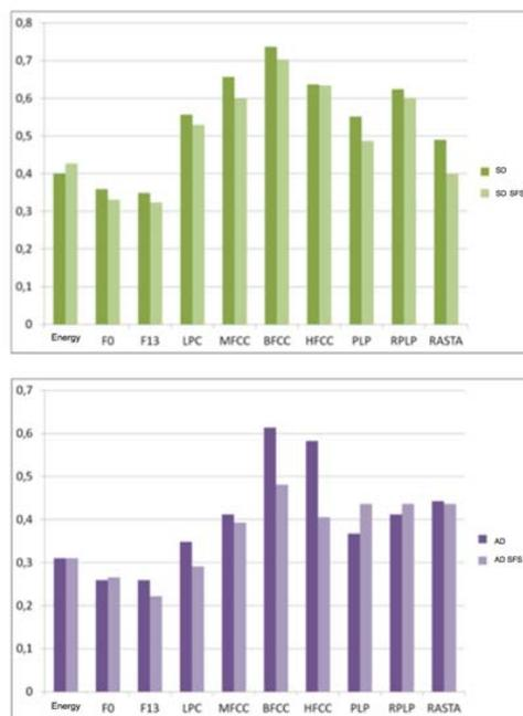
Fig.3. Errors value for each subset: top - Spontaneous Database SB, bottom Acted out Database AD
