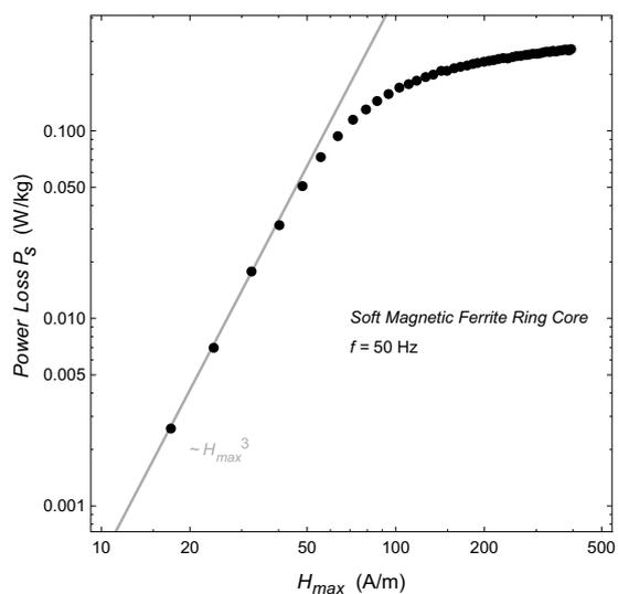
Fig.4. Log-log plot of the total weight specific power loss  $P_s$  in dependence on the field amplitude  $H_{max}$  of a soft magnetic ferrite ring core specimen. Note the increase of  $P_s$  with  $H_{max}^3$  for small values of  $H_{max}$  (solid line).
