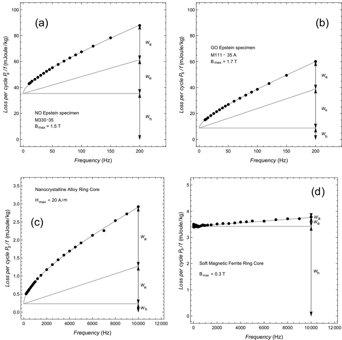
Fig.3. Examples of the separation of loss per cycle in dependence on the frequency for four different specimens of soft magnetic material.
