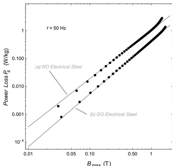
Fig.5. Log-log plot of the total weight specific power loss  $P_s$  of minor loops in dependence on their flux density amplitude  $B_{max}$  of a non-oriented electrical steel Epstein specimen (a) and of a grain-oriented electrical steel Epstein specimen (b). Note the increase of  $P_s$  with  $B_{max}^p$  in both cases for a broad range of flux density amplitudes indicated by the straight solid lines.
