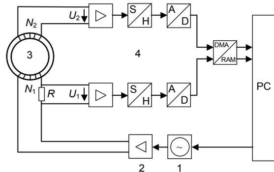
Fig. 1. Operating principle of the REMACOMP<sup>®</sup> C BH-loop tracers: 1 programmable signal generator, 2 power amplifier, 3 specimen with a primary winding of  $N_1$  turns and a secondary winding of  $N_2$  turns, 4 data acquisition system: digital sampling system with preamplifiers and analog/digital converters.
