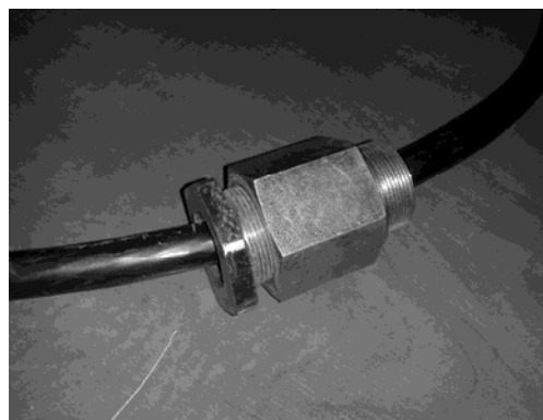
Fig. 1. Cable gland W1 – ferromagnetic material [2]
