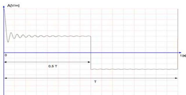
Fig. 1. The course of the electrical component of the electromagnetic field emitted by the monitor [1]
