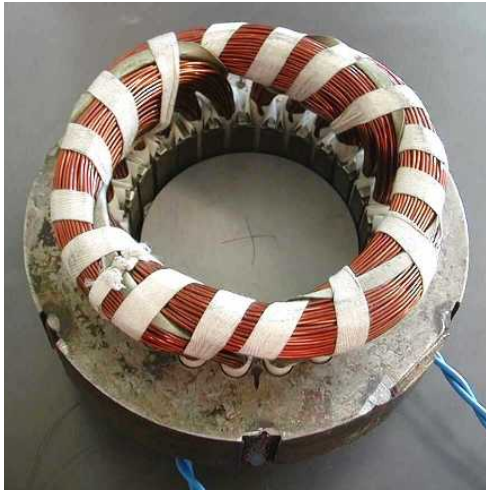
Fig.3. Two-phase yoke for rotational magnetisation of a single-sheet sample [7]
