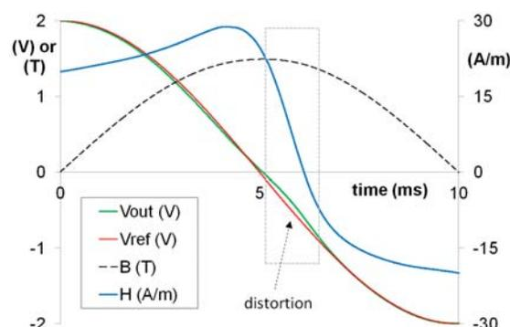
Fig.2. Signals recorded for a toroidal sample of grain-oriented electrical steel, magnetised at 1.55 T and 50 Hz, form factor of  $V_{out}$  diverged by 0.99%; only half-cycle is shown for clarity
