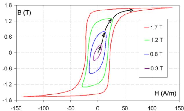
Fig.3. Maximum target value must pass through all the intermediate values
