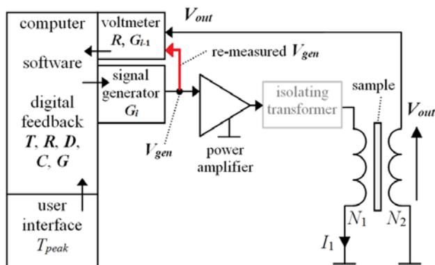
Fig.7. Block diagram of magnetising setup with DF:  $R$  corresponds to  $V_{out}$  and  $G$  to  $V_{gen}$
