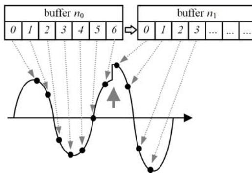
Fig.9. Explanation of the mechanism behind current glitches
