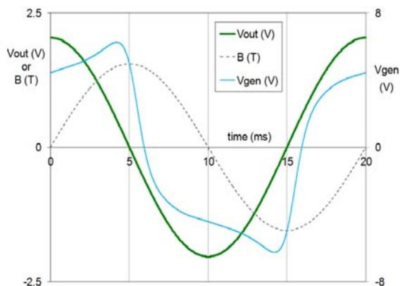
Fig.8. Typical phase relationship for secondary voltage "Vout", flux density "B", and generated voltage "Vgen"
