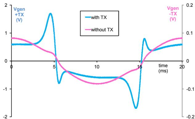
Fig.12.  $V_{gen}$  with (+TX) and without (-TX) the isolating transformer
