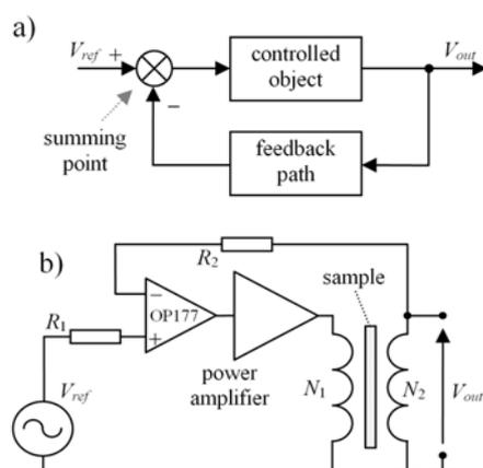
Fig.1. Analogue electronic feedback: a) block diagram of a system with a negative feedback loop, b) implementation with operational amplifier and power amplifier;  $R_1 = R_2 = 4.7 \text{ k}\Omega$ ; power supplies and decoupling power supply capacitors are not shown for OP177
