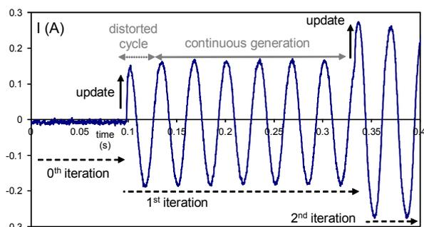
Fig.4. Magnetising current through initial iterations
