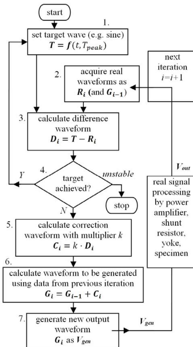
Fig.6. Digital feedback algorithm,  $i$  – iteration
