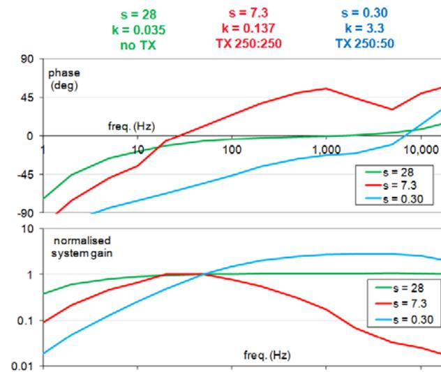
Fig.13. Phase (top) and gain (bottom) characteristics for:  $s = 28$  ( $k < 0.035$ ) without transformer,  $s = 7.3$  ( $k < 0.137$ ) with transformer 250:250, and  $s = 0.30$  ( $k < 3.3$ ) with transformer 250:50; gain curves normalised to 50 Hz
