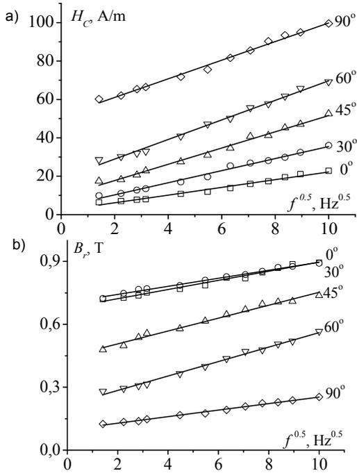
Fig. 2. Coercivity  $H_C^x$  (a) and remanence  $B_r^x$  (b) versus frequency  $\sqrt{f}$  for GO grade M140-30N at  $B_m = 1.0$  T
