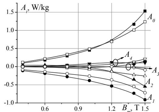
Fig. 5. Variation of coefficients  $A_i$  of (5) versus flux density  $B_m$  at 50 Hz for sample M140-30S, filled symbols hysteresis  $P_{h,y}^x$  and empty symbols additional eddy current  $P_{a,y}^x$  specific loss components [7].
