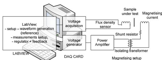
Fig. 1. The block diagram of measuring system [6, 7].
