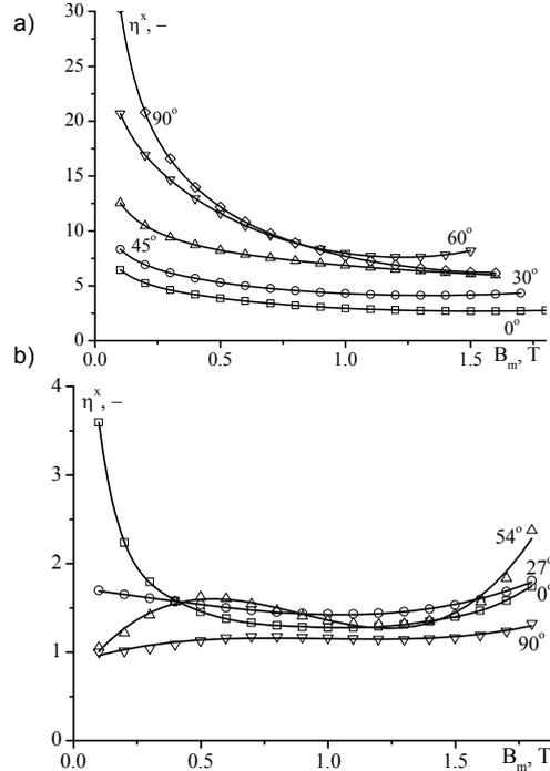
Fig. 3. Angular dependence of additional eddy current loss factor  $\eta^x$  versus maximum flux density  $B_m$  in a) GO ES grade M140-30N and b) NO ES grade M400-35S
