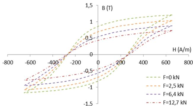
Figure 8. Magnetic hysteresis loops of the sample magnetic circuit, under various mechanical loads for second configuration.  $H$  - magnetizing field;  $B$  - flux density,  $F$  - force
