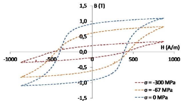
Figure 5. Magnetic hysteresis loops of the compressed sample under various mechanical loads for first configuration. H - magnetizing field, B - flux density,  $\sigma$  - compressive stress
