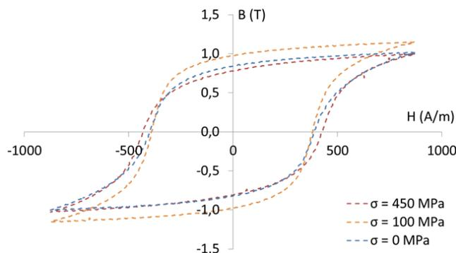
Figure 6. Magnetic hysteresis loops of the stretched sample under various mechanical loads for first configuration. H - magnetizing field, B - flux density,  $\sigma$  - tensile stress
