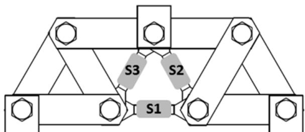
Fig. 2. Schematic diagram of the truss structures for first configuration, S1, S2, S3 - magnetic cores
