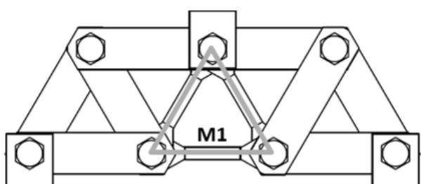
Fig. 3. Schematic diagram of the truss structures for second configuration, M1 - magnetic core
