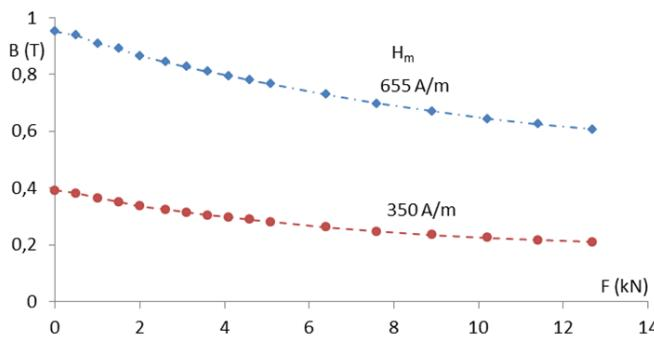
Figure 9. Magnetoelastic  $B(F)H$  characteristics for compressive and tensile stress for second configuration.  $F$  – force,  $B$  - flux density,  $H_m$  - magnetizing field
