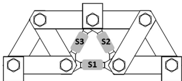
Fig. 2. Schematic diagram of the truss structures for first configuration, S1, S2, S3 - magnetic cores
