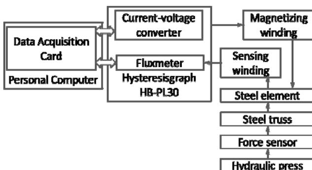
Fig. 1. Schematic block diagram of the test stand
