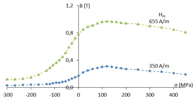
Figure 7. Magnetoelastic B(F)H characteristics for compressive and tensile stress for first configuration,  $\sigma$  - stress, B - flux density,  $H_m$  - magnetizing field
