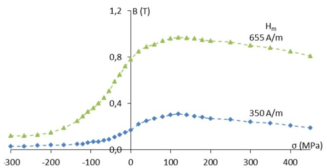
Figure 7. Magnetoelastic B(F)H characteristics for compressive and tensile stress for first configuration,  $\sigma$  – stress, B – flux density,  $H_m$  – magnetizing field
