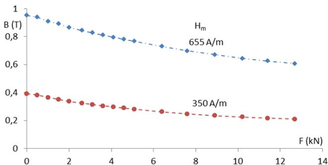
Figure 9. Magnetoelastic  $B(F)H$  characteristics for compressive and tensile stress for second configuration.  $F$  - force,  $B$  - flux density,  $H_m$  - magnetizing field
