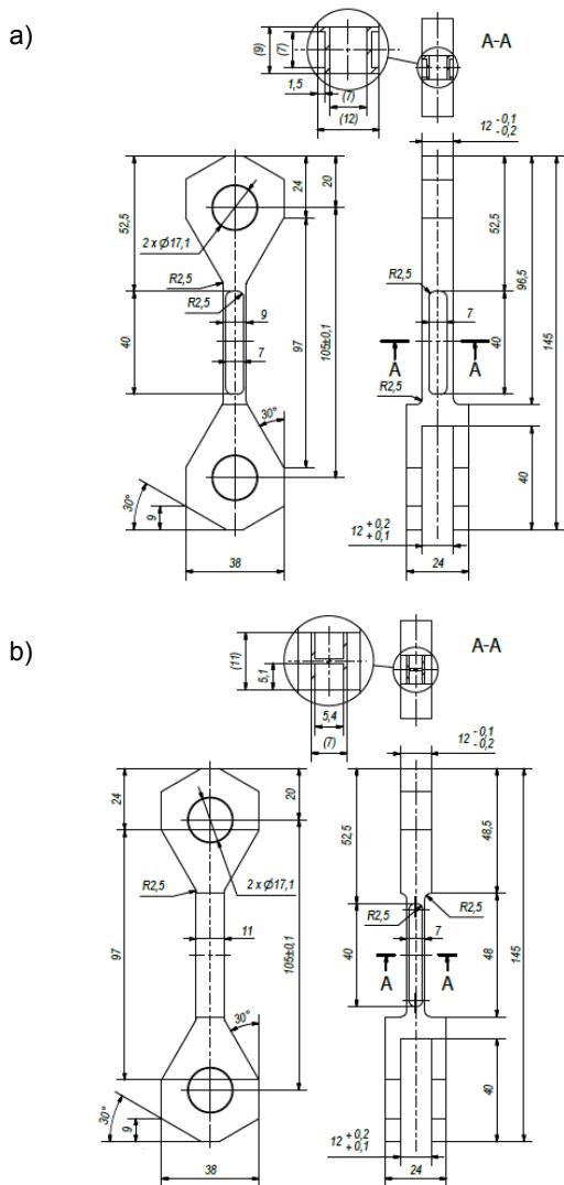
Fig. 4. Schematic diagram of the sample members
