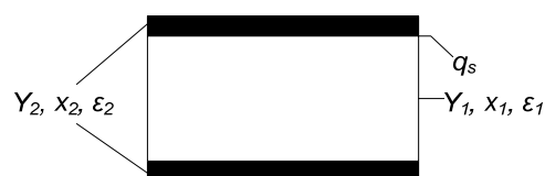
Fig. 1. Model of a layered dielectric structure containing charges with densities of +q_s and -q_s on the interfaces between the layers
