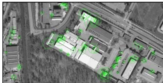
Fig.3. The detection of the key points by Speeded-Up Robust Features (SURF).
