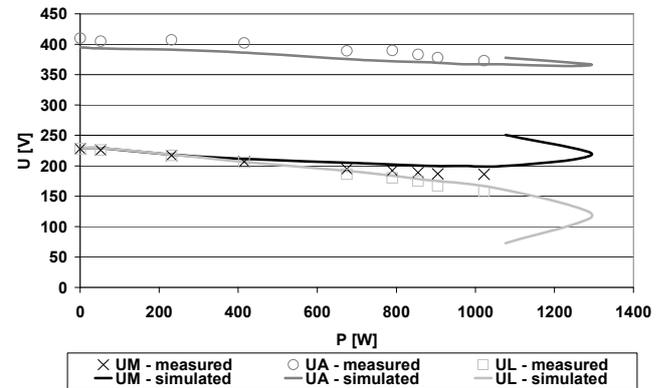
Fig. 9. Voltages versus output power of the SPSEIG with short-shunt capacitor topology in load stator winding
