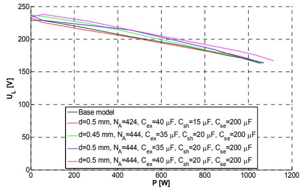
Fig. 5. Terminal voltage ( $U_L$ ) versus output power of the SPSEIG with short-shunt capacitors in load stator winding
