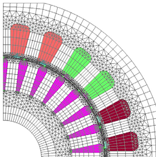
Figure 1. FE mesh of 2D field-circuit model of the SPSEIG
