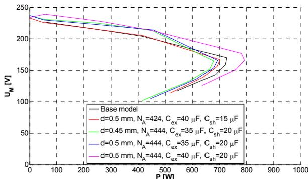
Fig. 3. Terminal voltage ( $U_M$ ) versus output power of the SPSEIG with shunt capacitor in load stator winding
