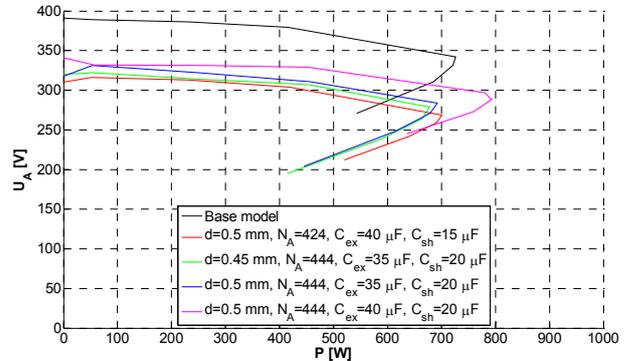
Fig. 4. Voltage of excitation stator winding ( $U_A$ ) versus output power of the SPSEIG with shunt capacitor in load stator winding
