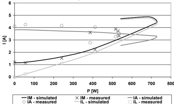
Fig. 8. Currents versus output power of the SPSEIG with shunt capacitor in load stator winding
