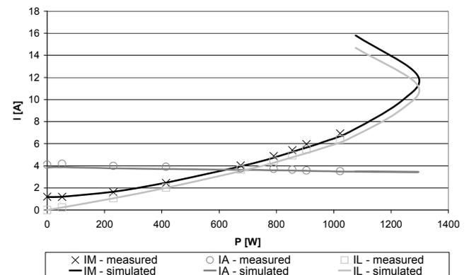
Fig. 10. Currents versus output power of the SPSEIG with short-shunt capacitor topology in load stator winding
