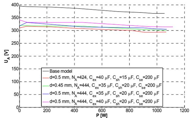
Fig. 6 Voltage of excitation stator winding ( $U_A$ ) versus output power of the SPSEIG with short-shunt capacitors in load stator winding
