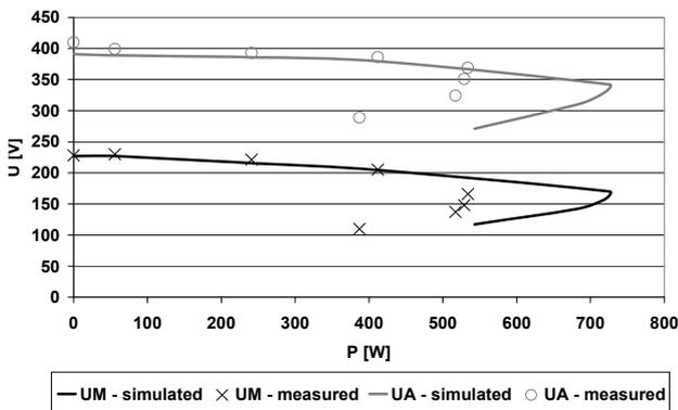
Fig. 7. Voltages versus output power of the SPSEIG with shunt capacitor in load stator winding
