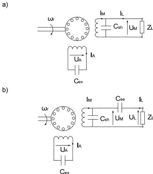
Fig. 2 Capacitor topology in the load stator winding: a) shunt connection, b) short-shunt connection
