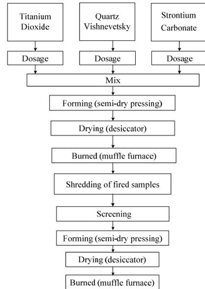
Fig. 3. Technological scheme for production of prototypes
