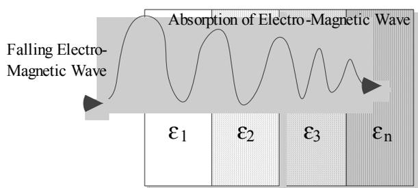
Fig. 1. Schematic view of the gradient radio-absorbing material
