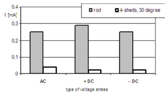
Fig.4. Average values of leakage currents recorded on 4-shed insulators with the inclination degree of upper surfaces of sheds equal to 30 degrees and on the insulator without sheds on the 7th day of ageing in the fog chamber at AC and DC voltage with both polarities.
