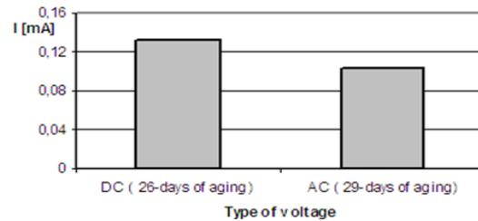
Fig.7. Comparison of daily average values of leakage current measured on the insulators subjected to the ageing process in the fog chamber at high DC and AC voltage.
