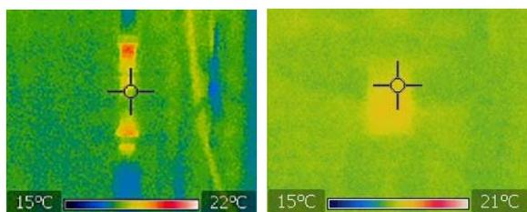
Fig.10. Temperature distribution along the surface of the insulator with sheds inclined at 0 degrees – 26 day of the experiment.
