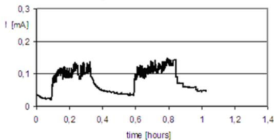
Fig.5. Leakage currents of 4-shed insulators with the inclination of the upper surfaces of 0 and 30 degrees on the 26th day of ageing in the fog chamber at DC voltage with positive polarity.
