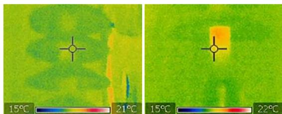
Fig.9. Temperature distribution along the surface of the insulator with sheds inclined at 30 degrees – 26 day of the experiment.
