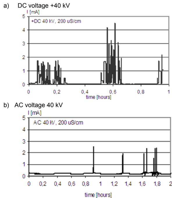
Fig.3. Leakage current for the insulators without sheds on the 6th day of the ageing process in the fog chamber: (a) insulators exposed to DC voltage with positive polarity, (b) insulators exposed to AC voltage.
