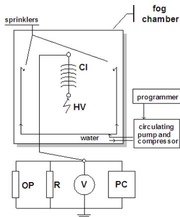
Fig.2. Diagram of the fog chamber. CI – composite insulator, OP – overvoltage protection device, V – voltmeter, PC – personal computer.
