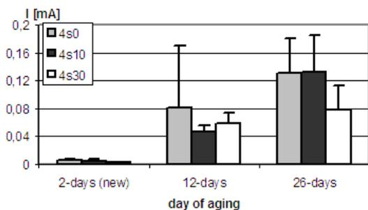
Fig.6. Comparison of daily average values of leakage currents measured on the second, twelfth and twenty-sixth day of ageing in the fog chamber.
