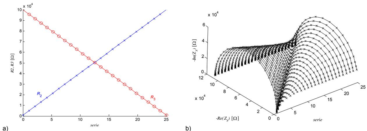
Fig. 3. Exemplary usage of model with impedance changing in time: a) resistor parameters change in mode 3, b) resulting DEIS diagram
