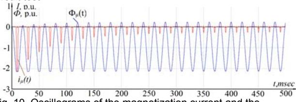
Fig. 10. Oscillograms of the magnetization current and the magnetic flux of  $\xi$ -phase of the SPT in on-load test
