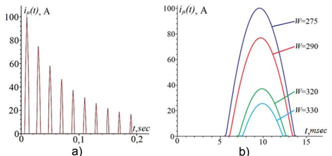
Fig. 5. Oscillograms of the magnetization current of the SPT in open-circuit test
