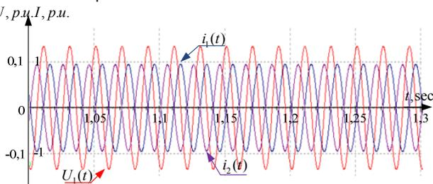
Fig. 9. Oscillograms of the current, voltage of primary winding and the current of secondary winding of  $\xi$ -phase of the SPT in short-circuit test
