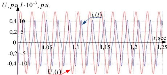
Fig. 7. Oscillograms of the current and voltage of  $\xi$ -phase primary winding of the SPT in open-circuit test
