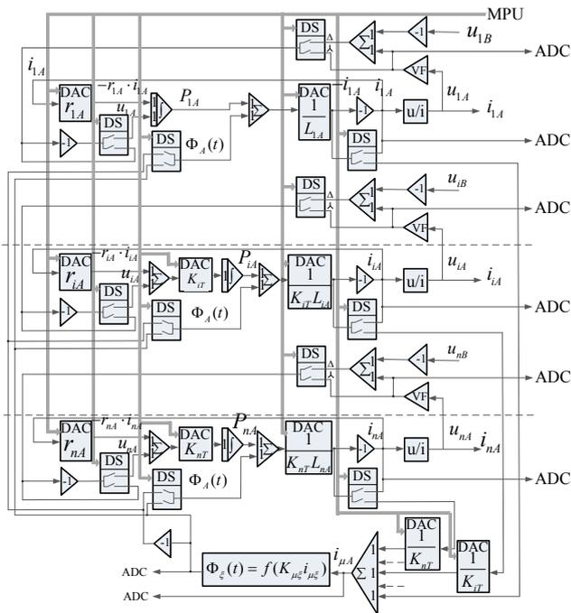
Fig. 2. The functional diagram for  $\xi=A$  (identical for  $\xi=B,C$ ) of HCP with  $n$ -windings of SPT: DAC – digital-to-analog converter; DS – digitally controlled three-phase switches; VF – voltage follower
