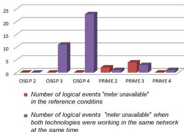
Fig.6. The results obtained for "meter unavailable" in relation to 1-hour testing
