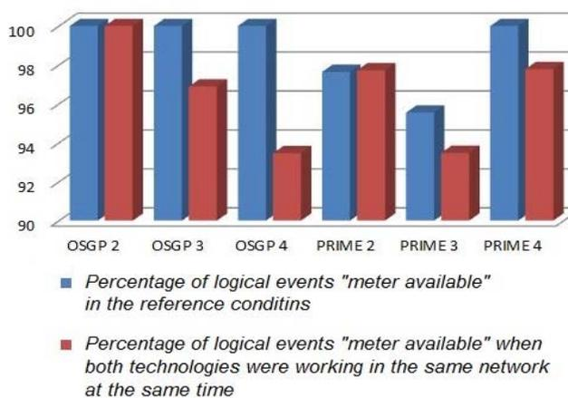
Fig.5. The results obtained for "meter available" in relation to 1-hour testing
