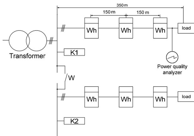
Fig.4. Scheme of the measurement system used in the experiment, where Wh-meter, K1, K2-concentrators
