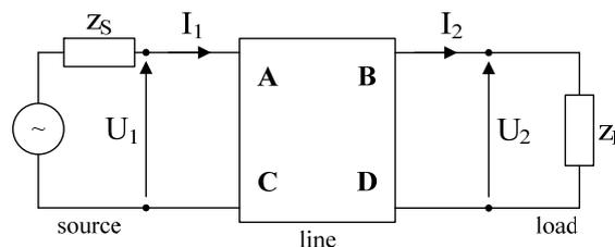
Fig.3. Simplified model of power supply line as a long line
