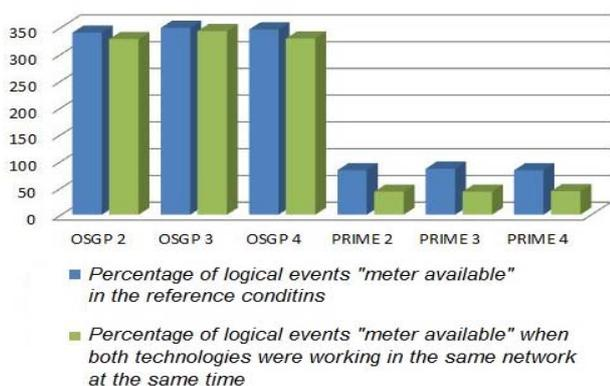
Fig.7. Comparative analysis of percentage transmission capacity of PLC technologies under investigation
