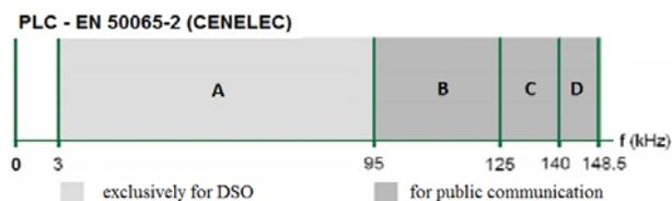
Fig.2. Frequencies in the CENELEC A band are used by various PLC technologies.
