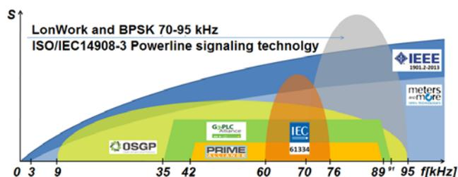
Fig.1. Frequency ranges dedicated for PLC transmission in compliance with EN 50065
