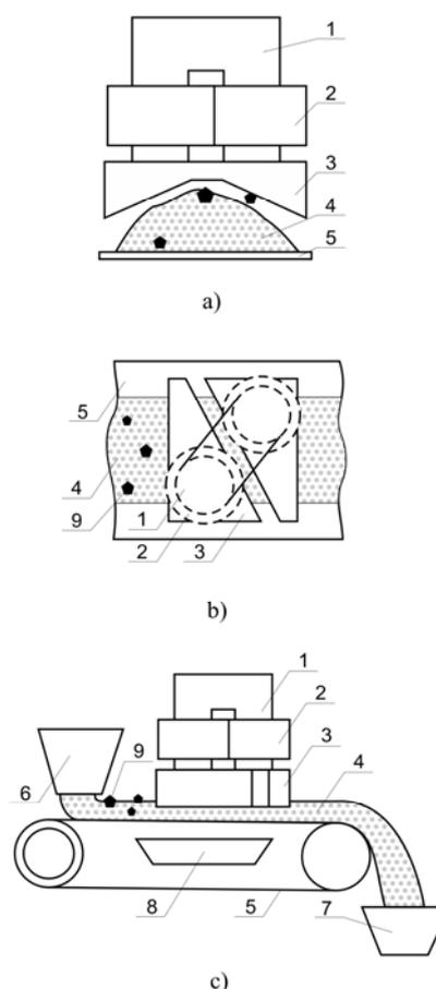
Fig. 1. Suspended electromagnetic iron separator with arch-shaped pole pieces (a – view along the conveyor belt; b – top view; c – overview), where 1 – magnetic system; 2 – magnetizing coil; 3 – pole piece; 4 – separated material; 5 – conveyor belt; 6 – initial material bunker; 7 – purified material bunker; 8 – bunker for the extracted ferromagnetic bodies; 9 – ferromagnetic bodies
