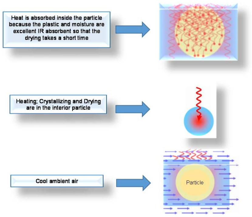
Fig.4. Process of drying material – IRD
