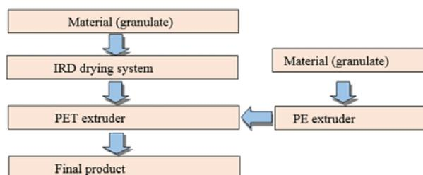
Fig.1. The concept of co-extrusion line for extruding PET sheets and products from these sheets
