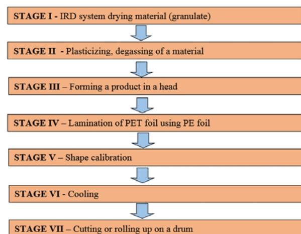
Fig.2. The stages of co-extrusion technological line for extruding PET sheets and products from these sheets
