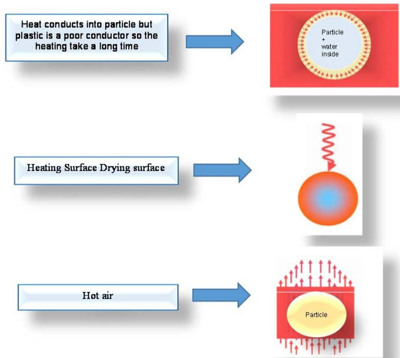
Fig.5. Process of conventional drying [10]
