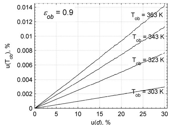
Figure 10: Component of the relative combined standard uncertainty associated with camera-to-object-distance  $d$  (results of simulations for data collected in table 1)
