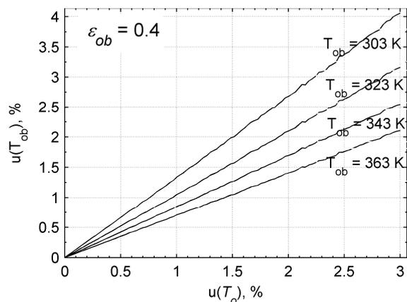
Figure 5: Component of the relative combined standard uncertainty associated with the ambient temperature  $T_o$  (results of simulations for data collected in table 1)
