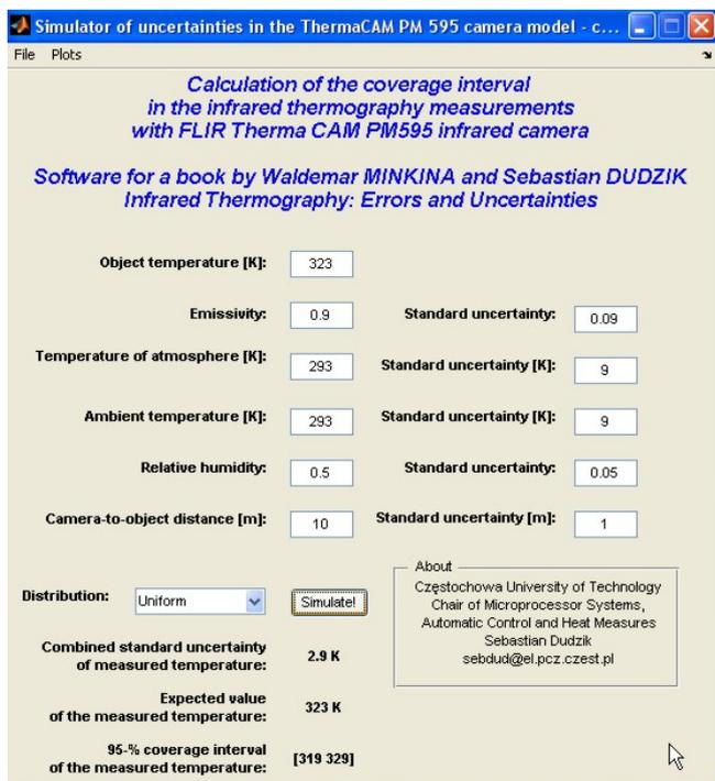
Figure 11: The main window screen shot of the program used for the calculations of the combined standard uncertainty in the temperature measurements with the FLIR ThermoCAM PM595 infrared camera
