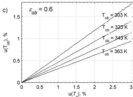
Figure 6: Component of the relative combined standard uncertainty associated with the ambient temperature  $T_o$  (results of simulations for data collected in table 1)
