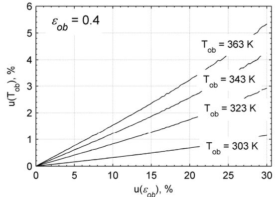
Figure 2: Component of the relative combined standard uncertainty associated with emissivity  $\epsilon_{ob}$  (results of simulations for data collected in table 1)
