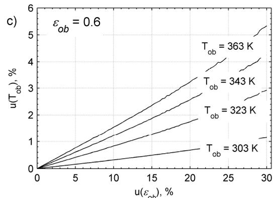
Figure 3: Component of the relative combined standard uncertainty associated with emissivity  $\epsilon_{ob}$  (results of simulations for data collected in table 1)
