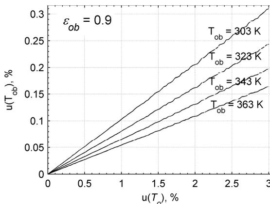
Figure 7: Component of the relative combined standard uncertainty associated with the ambient temperature  $T_o$  (results of simulations for data collected in table 1)
