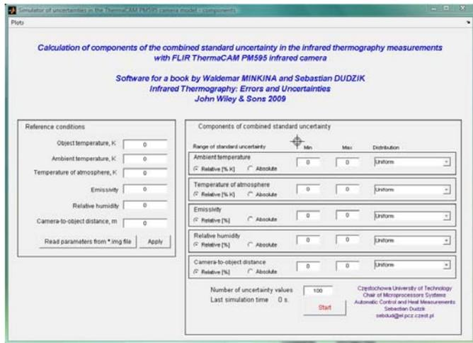
Figure 1: The main window screenshot of the program used for the calculations of the components of combined standard uncertainty in the measurements with the FLIR ThermoCAM PM595 infrared camera
