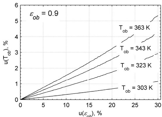
Figure 4: Component of the relative combined standard uncertainty associated with emissivity  $\epsilon_{ob}$  (results of simulations for data collected in table 1)
