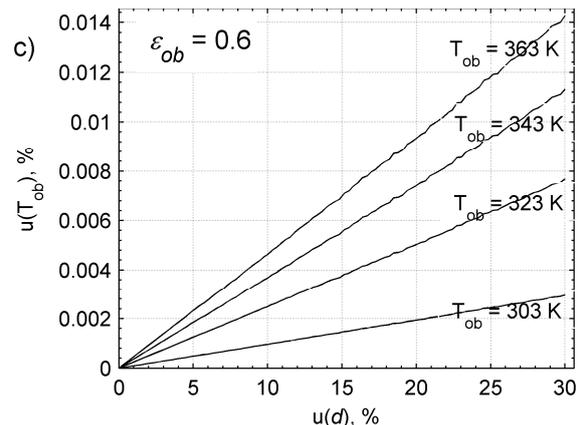
Figure 9: Component of the relative combined standard uncertainty associated with camera-to-object-distance  $d$  (results of simulations for data collected in table 1)
