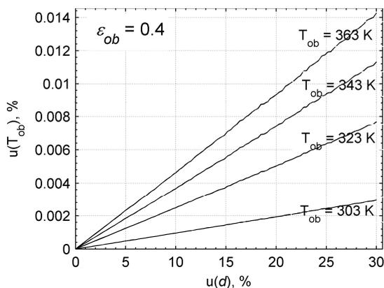
Figure 8: Component of the relative combined standard uncertainty associated with camera-to-object-distance  $d$  (results of simulations for data collected in table 1)
