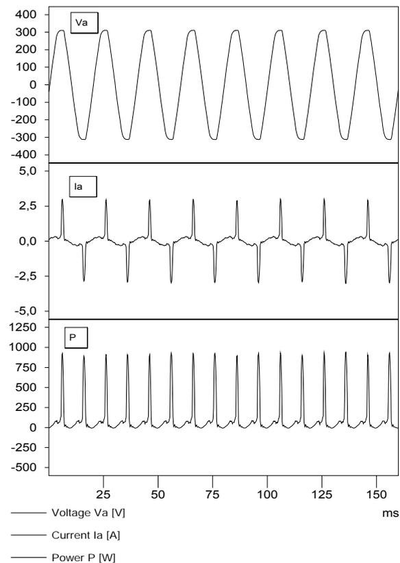
Fig. 4. The time characteristics of the supply voltage, the supply current and the active power of the Kawasaki robot at the static state
