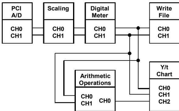
Fig. 3. The block diagram of the voltage and current measurement signal processing system of the Kawasaki FS03N robot
