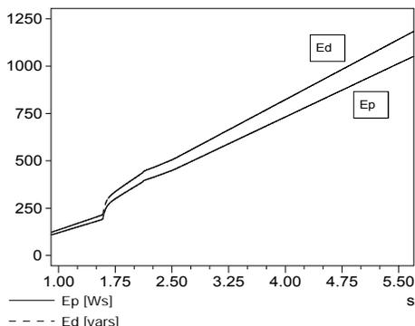
Fig. 7. The time characteristics of active energy and distortion reactive energy of the Kawasaki robot at moving the JT1 axis
