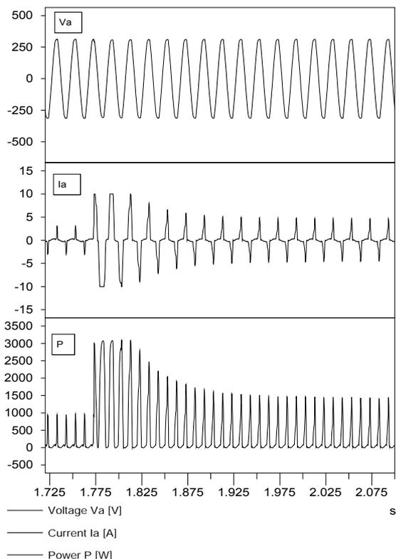
Fig. 6. The time characteristics of the supply voltage, the supply current and the active power of the Kawasaki robot at moving the JT2 axis
