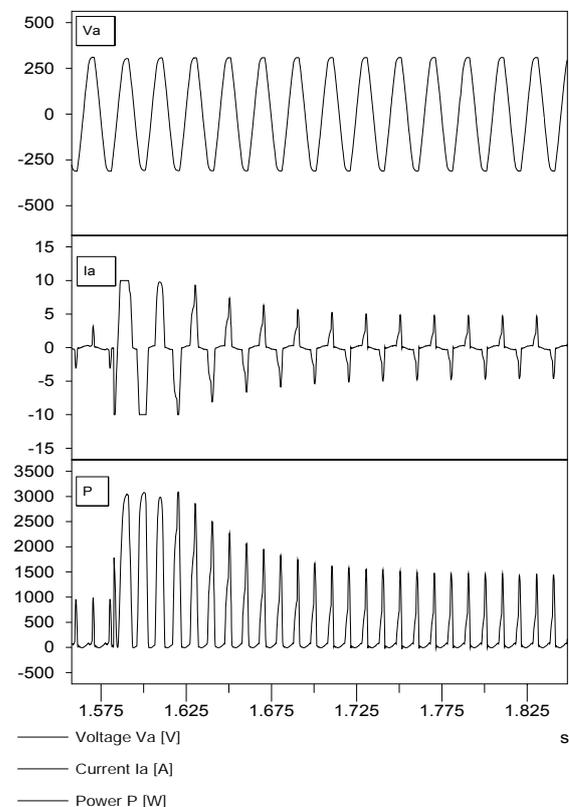
Fig. 5. The time characteristics of the supply voltage, the supply current and the active power of the Kawasaki robot at moving the JT1 axis
