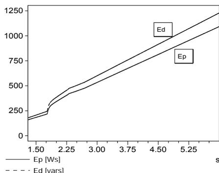
Fig. 8. The time characteristics of active energy and distortion reactive energy of the Kawasaki robot at moving the JT2 axis
