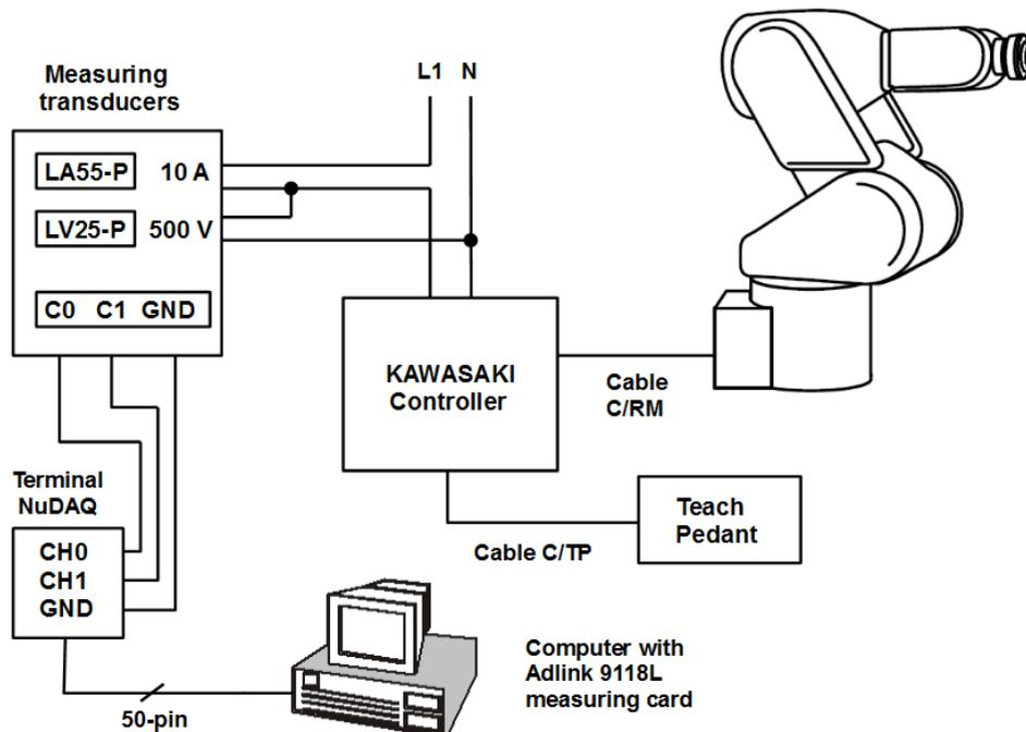
Fig. 2. The block diagram of the computer measuring system for voltage and current of the Kawasaki FS03N robot
