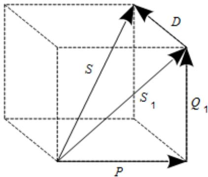
Fig. 1. The power component vectors of the non-linear receiver [2]
