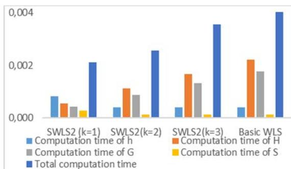
Fig.12. Computation time details in seconds for SWLS2 algorithm applied to IEEE14 bus system
