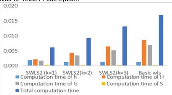
Fig.13. Computation time details in seconds for SWLS2 algorithm applied to IEEE30 bus system
