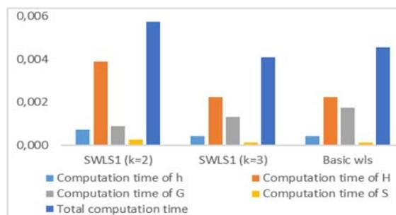
Fig.9. Computation time details in seconds for SWLS1 algorithm applied to IEEE14 bus system
