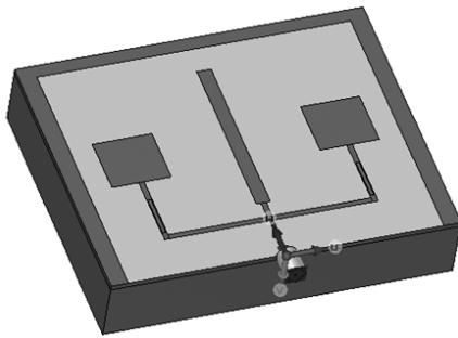
Fig.3. Antenna used in EMF exposure system
