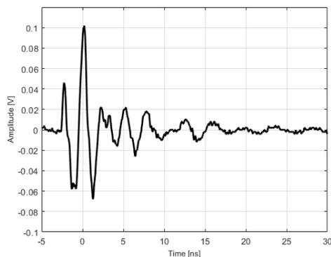
Fig. 7. Time characteristic - test 1 with a fibre-optic link
