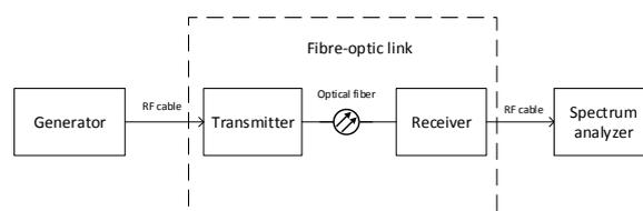
Fig. 1. Block diagram of a laboratory test stand for the determination of the frequency and transfer characteristics.
