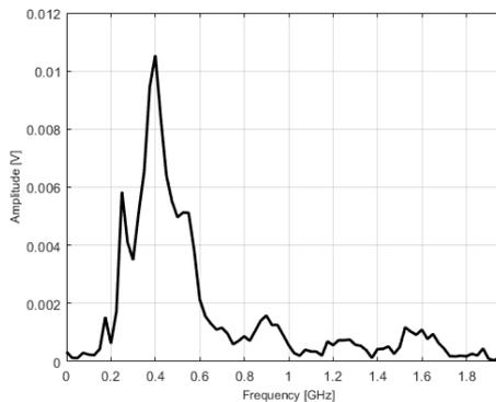
Fig. 12. Signal spectrum - test 2 with fibre-optic link
