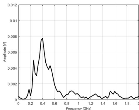
Fig.14. Signal spectrum – test 2 without fibre-optic link
