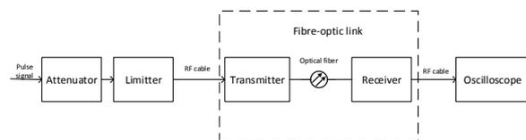
Fig. 3. Block diagram of a laboratory test stand for recording the output signal
