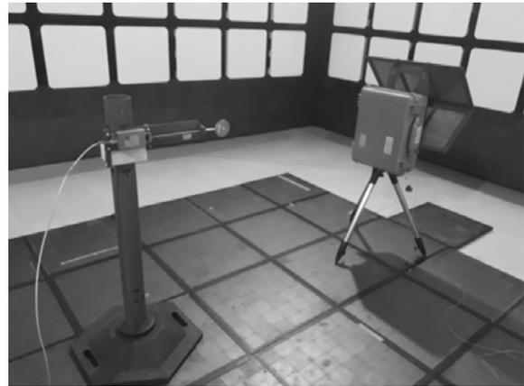
Fig. 4. Pulsed electromagnetic field generator with a D-dot probe and a balun
