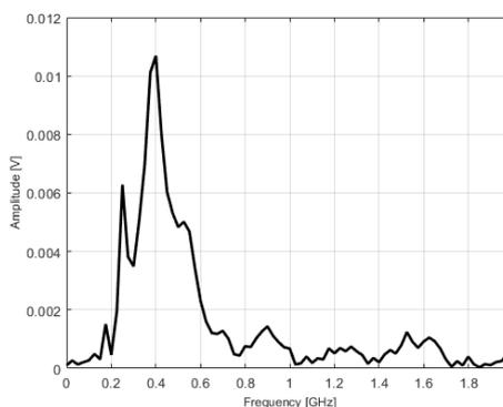
Fig. 11. Signal spectrum - test 1 with fibre-optic link
