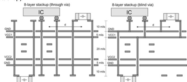
Fig. 10. Capacitor placement for 8-layer stackup.
