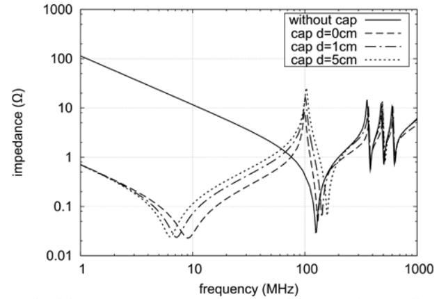
Fig. 3. PDN impedance for different distances between IC and decoupling capacitor (four layers stackup with 35 mils between planes).
