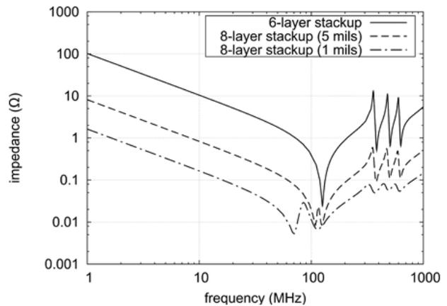
Fig. 8. PDN impedance for the three analyzed layer stackups.
