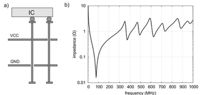
Fig. 1. A 4-layer stackup (a) and frequency behaviour of power planes (b).
