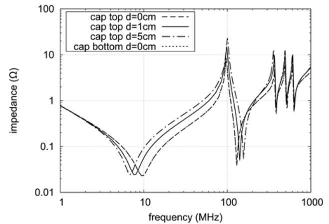
Fig. 9. PDN impedance for different capacitor placement (6-layer stackup).
