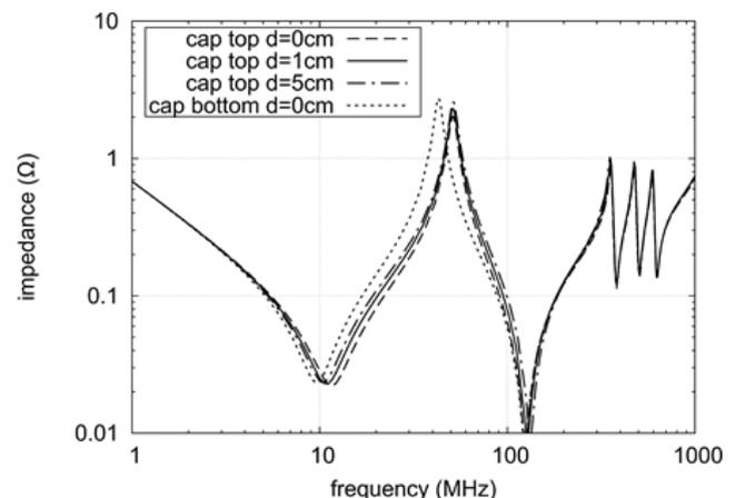
Fig. 11. PDN impedance for different capacitor placement (8-layer stackup, through via).
