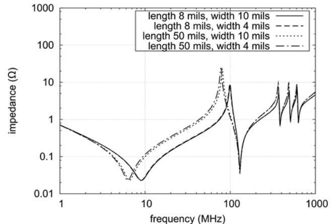
Fig. 5. PDN impedance for different capacitor mounting (capacitor close to the IC, four layers stackup with 35 mils between planes).
