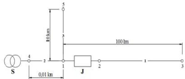
Fig.3. Diagram of power network computational structure
