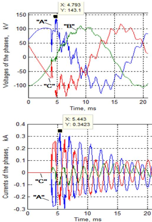
Fig.4. Voltage ( $U_{1MAX}$ ) value in the first node, and current ( $I_{1MAX}$ ) value in the first line. Circuit breaker operation from the stationary regime, and all phases are simultaneously activated
