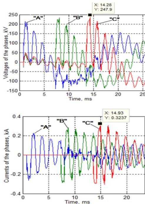
Fig.6. Voltage ( $U_{3MAX}$ ) value in the third node, and current ( $I_{1MAX}$ ) value in the first line. Circuit breaker operation from the stationary regime, and all phases are not simultaneously activated
