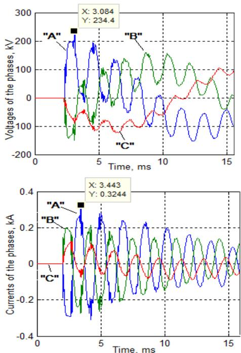
Fig.5. Voltage ( $U_{3MAX}$ ) value in the third node, and current ( $I_{1MAX}$ ) value in the first line. Circuit breaker operation from the stationary regime, and all phases are simultaneously activated
