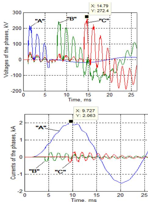
Fig.7. Voltage ( $U_{3MAX}$ ) value in the third node, and current ( $I_{1MAX}$ ) value in the first line during single phase fault. All phases are not simultaneously activated
