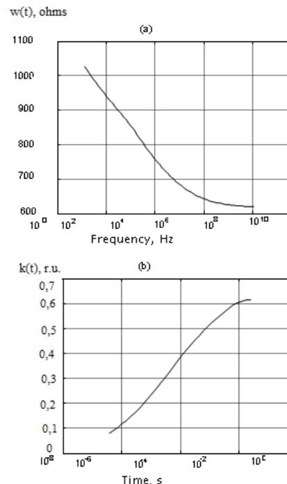
Fig.2. Surge impedance's real frequency function (a) and change in time factor (b)
