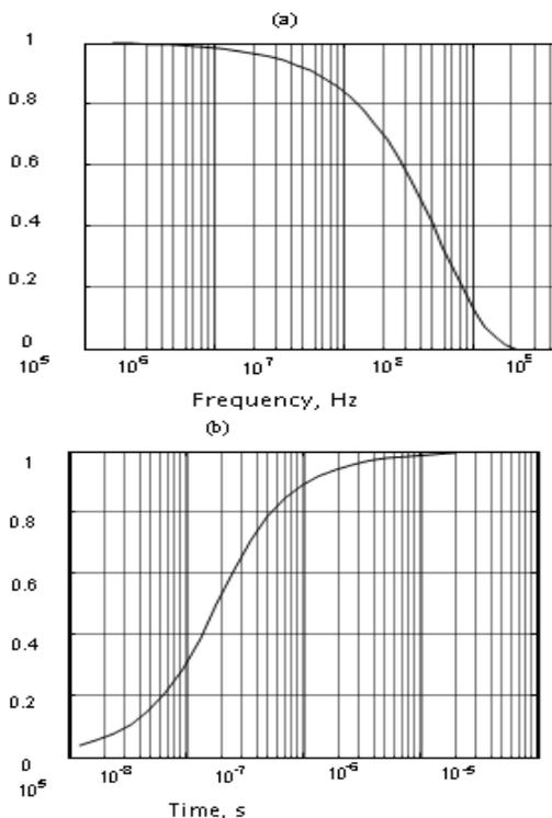
Fig.1. Electromagnetic wave suppression's real frequency function (a) and in time function (b)
