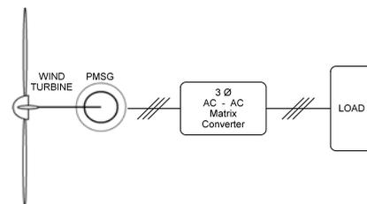
Fig.4. Matrix Converter based Wind Energy Conversion System
