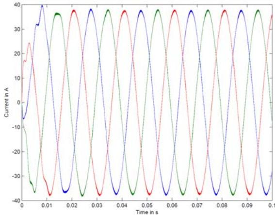
Fig.20. Output load current waveform for 50% load
