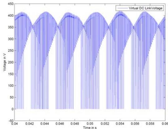
Fig. 14. Virtual DC link voltage waveform for time period 40ms to 60ms
