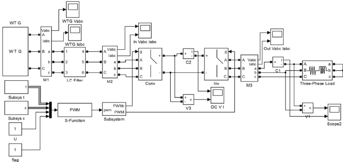
Fig. 8. PMSG based standalone WECS Simulink model using Two Stage Matrix Converter
