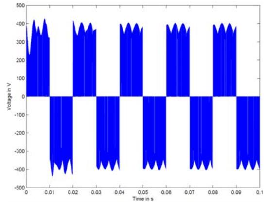
Fig. 17. Line-line output load voltage waveform of  $V_{AB}$
