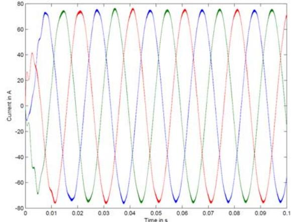
Fig.24. Output load current waveform for full load
