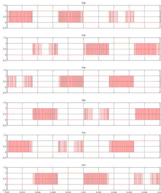
Fig. 12. VSR-TSMC three leg switching pulse for time period 20ms to 40ms
