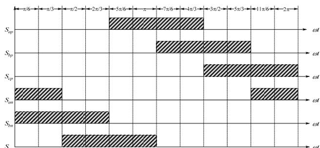
Fig.6. Switching waveforms of the voltage source rectifier
