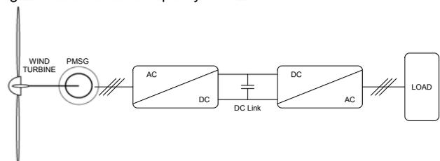
Fig.3. Conventional AC – DC – AC conversion system
