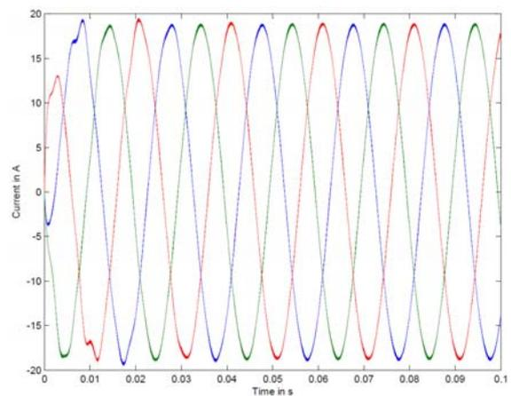
Fig. 18. Output load current waveform for 25% load
