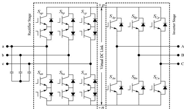
Fig.5. Schematic view of Two Stage Matrix Converter (TSMC)
