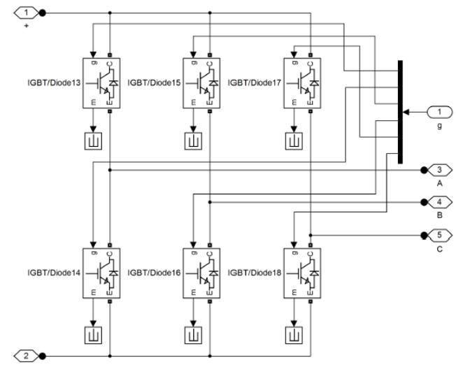
Fig. 11. Current source inverter stage of TSMC
