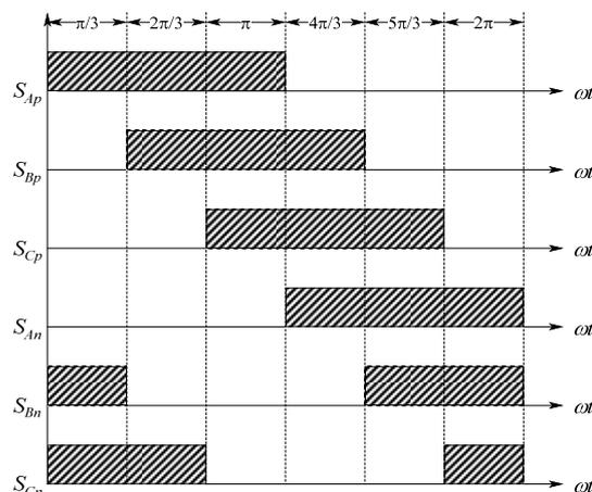
Fig.7. Switching waveforms of the current source inverter
