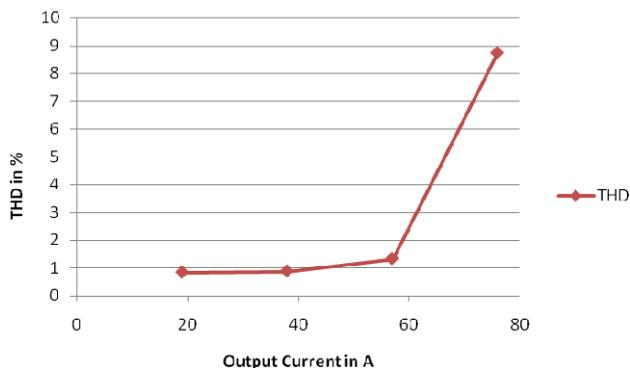
Fig.27. THD Vs load current
