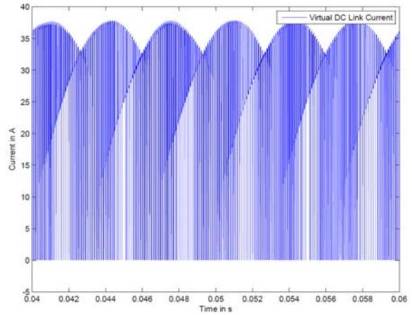
Fig. 15. Virtual DC link current waveform from time period 40ms to 60ms
