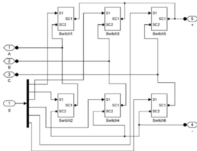
Fig. 9. Voltage source rectifier stage of TSMC
