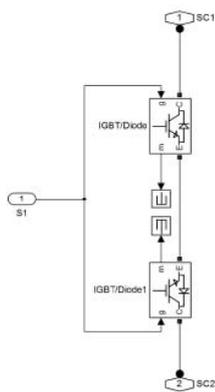
Fig. 10. Single bidirectional switch module of TSMC-voltage source rectifier
