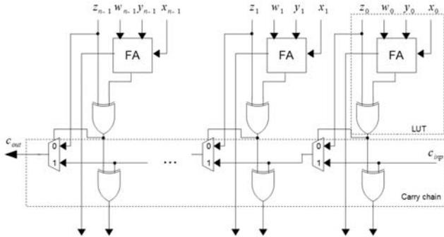
Fig.6. Xilinx FPGA realization of the 4-operand n-bit CSA type adder (based on Fig. 5)
