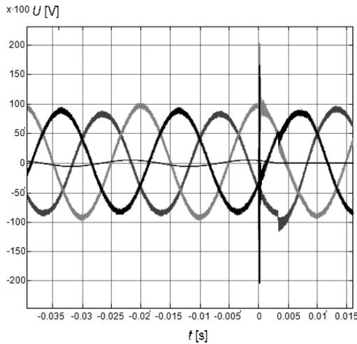
Fig. 7. Transient process of switching off of the reactor
