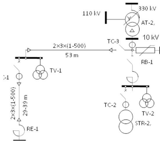
Fig. 2. Connection diagram of reactor
