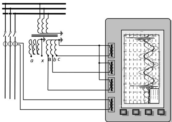
Fig 4. Scheme of connection of recorder
