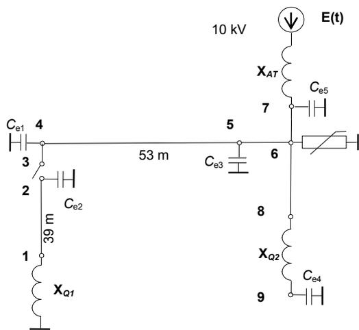
Fig. 3. Computational diagram of reactor connection
