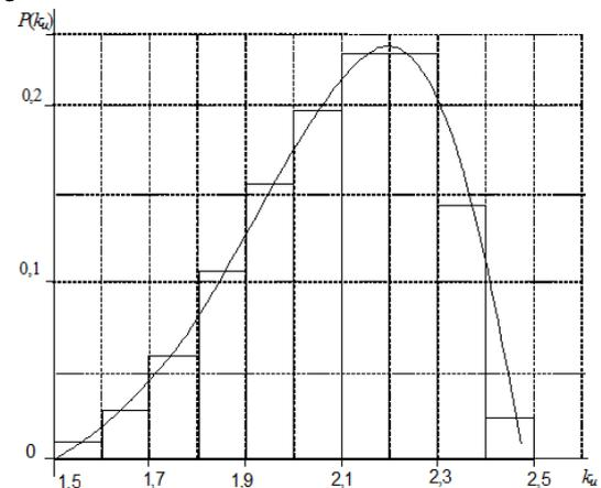
Fig. 10. Histogram of the level of overvoltages
