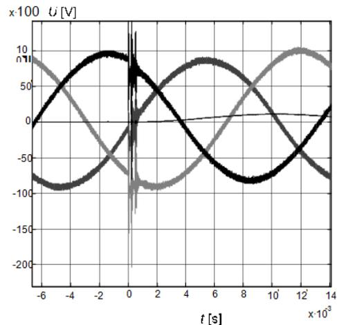
Fig. 5. Transient process of switching on of the reactor
