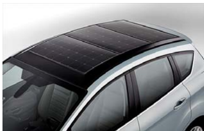
Fig.1. Roof of a car with solar modules and Fresnel system of lens [3]
