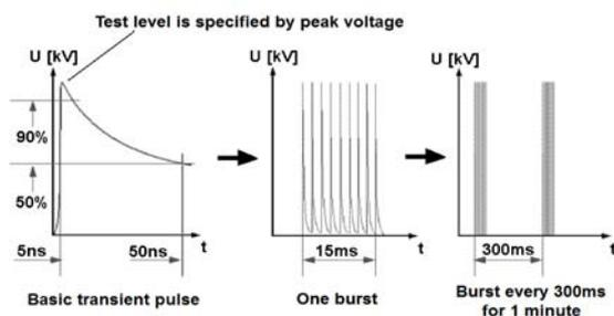
Fig.1. Standard EFT test waveform
