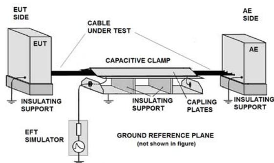
Fig.2. Test workplace arrangement with capacitive clamp
