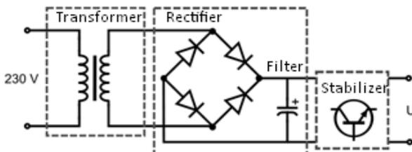
Fig. 1 Linear power supply diagram.
