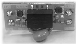
Fig. 22 Converter with isolated output.
