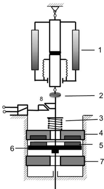
Fig. 2. Vacuum Switching Unit. 1 – vacuum interrupter, 2 – isolator, 3 – springs set, 4 – drive's coil, 5 – copper disc, 6 – base of disc, 7 – bumper, 8 - lock
