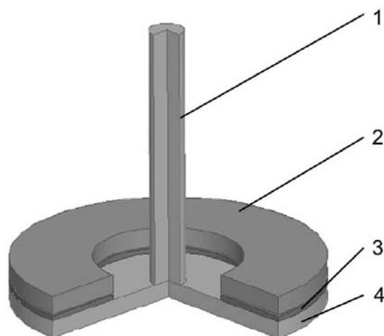
Fig. 3. Cross – section of 3D model of IDD. 1 – driving rod connecting movable contact with disc, 2 – drive's coil, 3 – disc, 4 – base of disc
