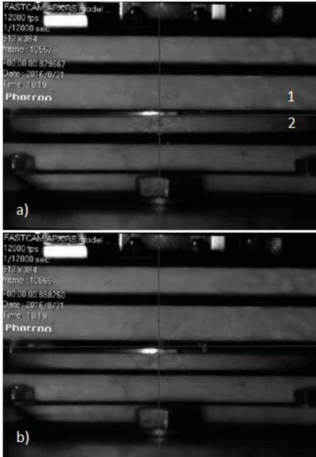
Fig. 9. Chosen frames from high-speed camera: a) Closed state, b) Opened state; 1 - coil, 2 - disc
