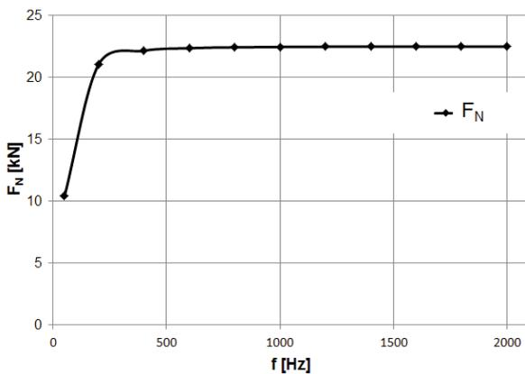
Fig. 6. The influence of frequency of coil's current  $f$  on repulsive force  $F_N$
