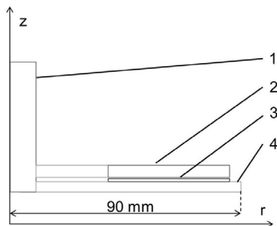
Fig. 4. 2D model of IDD defined in Ansoft Maxwell 2D. 1 – vacuum interrupter, 2 – isolator, 3 – springs set, 4 – drive's coil, 5 – copper disc, 6 – base of disc, 7 – bumper
