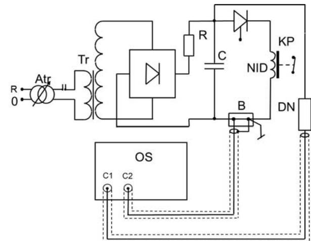
Fig. 8. Scheme of laboratory stand for Vacuum Switching Unit checking. NID - Inductive Dynamic Drive, KP - vacuum interrupter, OS - oscilloscope, B - Shunt, DN - voltage probe, C - capacitors, Atr - autotransformer, Tr - transformer, Pr - rectifier
