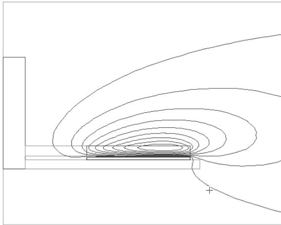
Fig. 5. Magnetic field distribution for frequency of coil's current equal to  $f = 2000$  Hz
