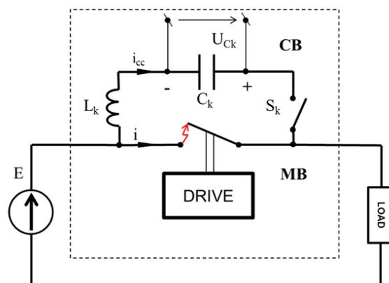
Fig. 1. Scheme of switch with force commutation . MB - main branch, CB - commutation branch
