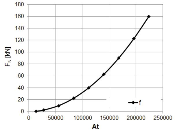
Fig. 7. The influence of a number of Ampere-turns on a maximal value of a repulsive force  $F_N$
