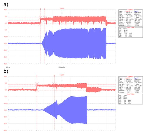
Fig.4. Control voltage signal of the HF generator (upper graphs) and the inductor current (lower graphs) for two cylinder speeds: 25 rpm (a) and 125 rpm (b)
