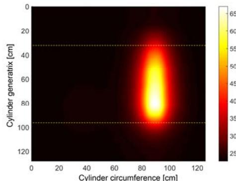
Fig.7. Temperature distribution at cylinder surface for two rotation speeds: 25 rpm (a) and 125 rpm (b), after correction of the heating circuit delay
