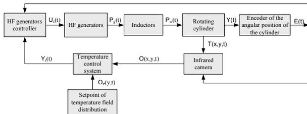
Fig.2. Block diagram of analysed part of the system
