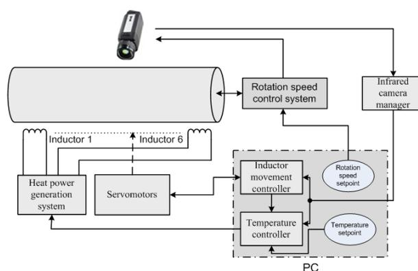
Fig. 1. Structure of the experimental setup
