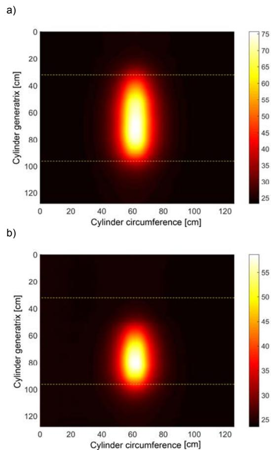
Fig.3. Temperature distribution at the cylinder surface for two values of rotation speed: 25 rpm (a) and 125 rpm (b)
