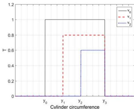
Fig.5. Simplified rectangular temperature profiles along a circumference of the cylinder (y coordinate) under different heating conditions
