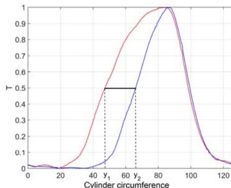
Fig.6. Determination of the equivalent delay of the heating channel
