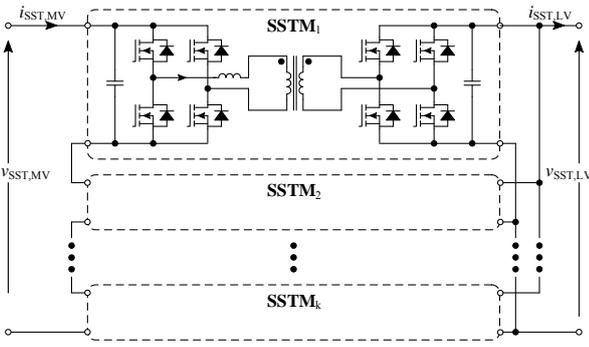
Fig. 1. Solid state transformer, SST, general concept. Built of input-series, output-parallel connected SST Modules, SSTM
