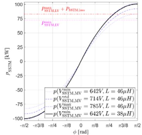
Fig. 3. The DAB converter power transfer characteristics for phase shift modulation, PSM, according to (1) as functions of  $\varphi_{SSTM,LV}$ . Plots drawn for  $V_{SSTM,LV} = 380$  V,  $V_{SSTM,MV}$  and  $L$  given in the plot legend. The inductance  $L = 38 \mu\text{H}$  was used in circuit considered in this paper
