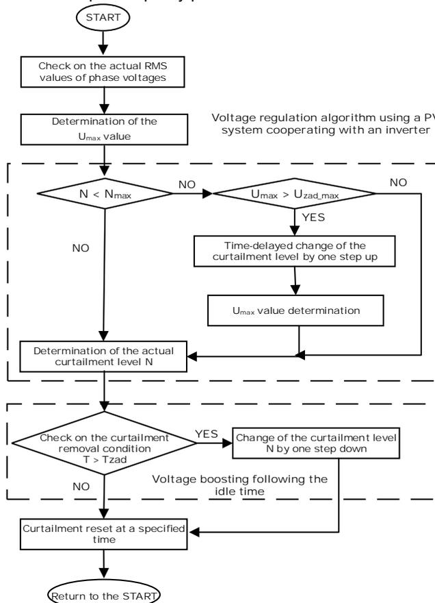
Fig. 2. Local control algorithm
