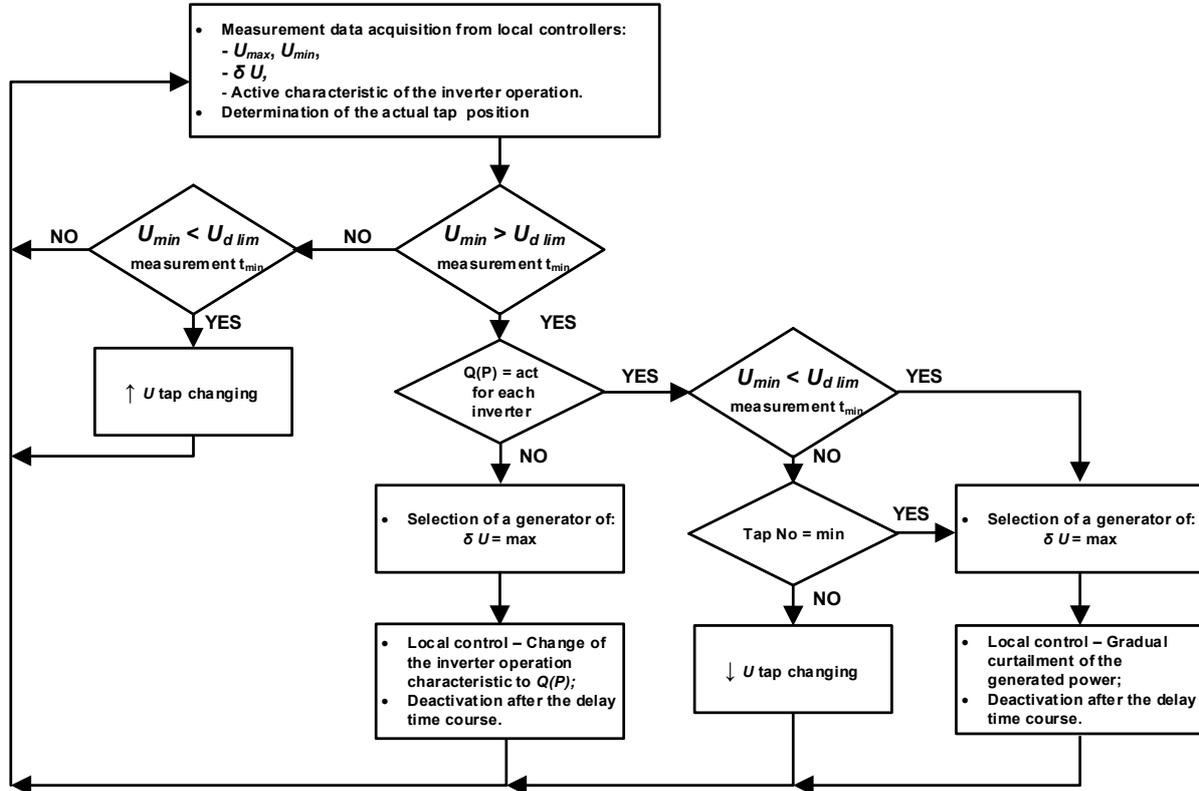
Fig. 4. Algorithm for distributed coordinated voltage control
