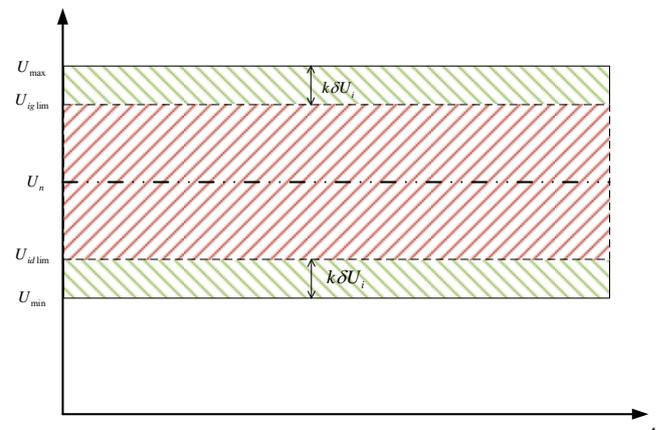
Fig. 3. Action ranges of the local and the distributed algorithms
